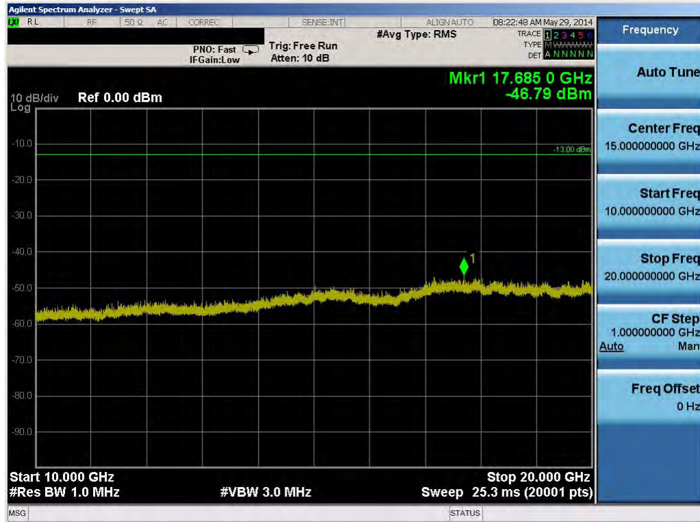
Plot 7-10. Conducted Spurious Plot (1.4MHz QPSK – RB Size 1, RB Offset 0 – High Channel)
