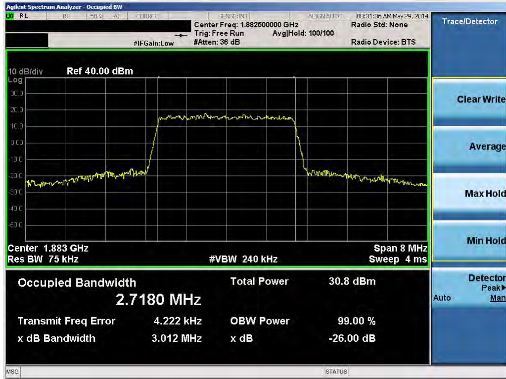
Plot 7-18. Occupied Bandwidth Plot (3.0MHz 16-QAM – RB Size 15)
