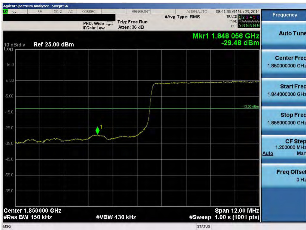
Plot 7-29. Lower Band Edge Plot (15.0MHz QPSK – RB Size 75)
