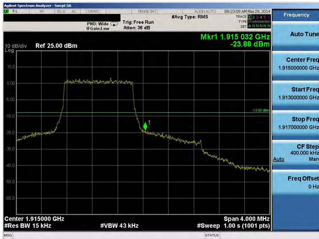
Plot 7-11. Upper Band Edge Plot (1.4MHz QPSK – RB Size 6)
