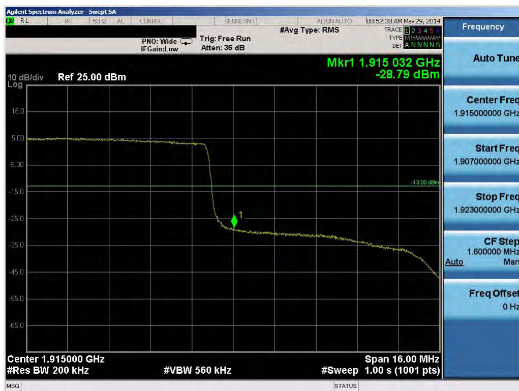
Plot 7-53. Upper Band Edge Plot (20.0MHz QPSK – RB Size 100)
