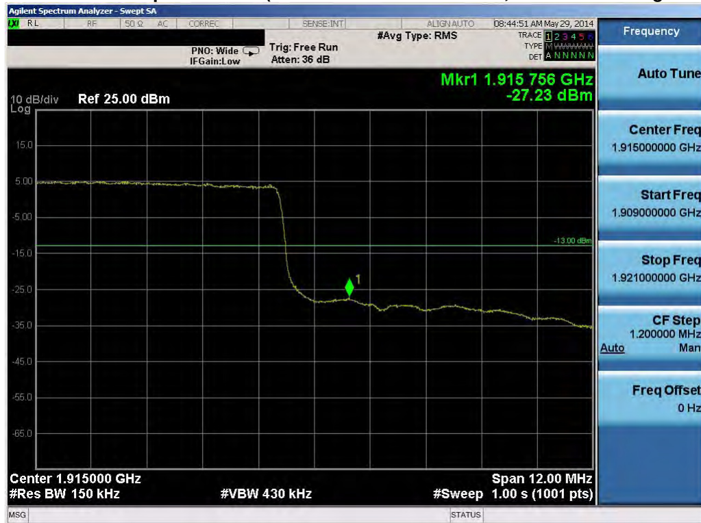
Plot 7-39. Upper Band Edge Plot (15.0MHz QPSK – RB Size 75)
