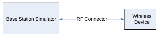
Figure 9-1 Power Measurement Setup
