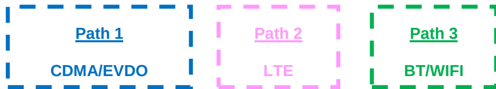
Figure 1-3 Simultaneous Transmission Paths
