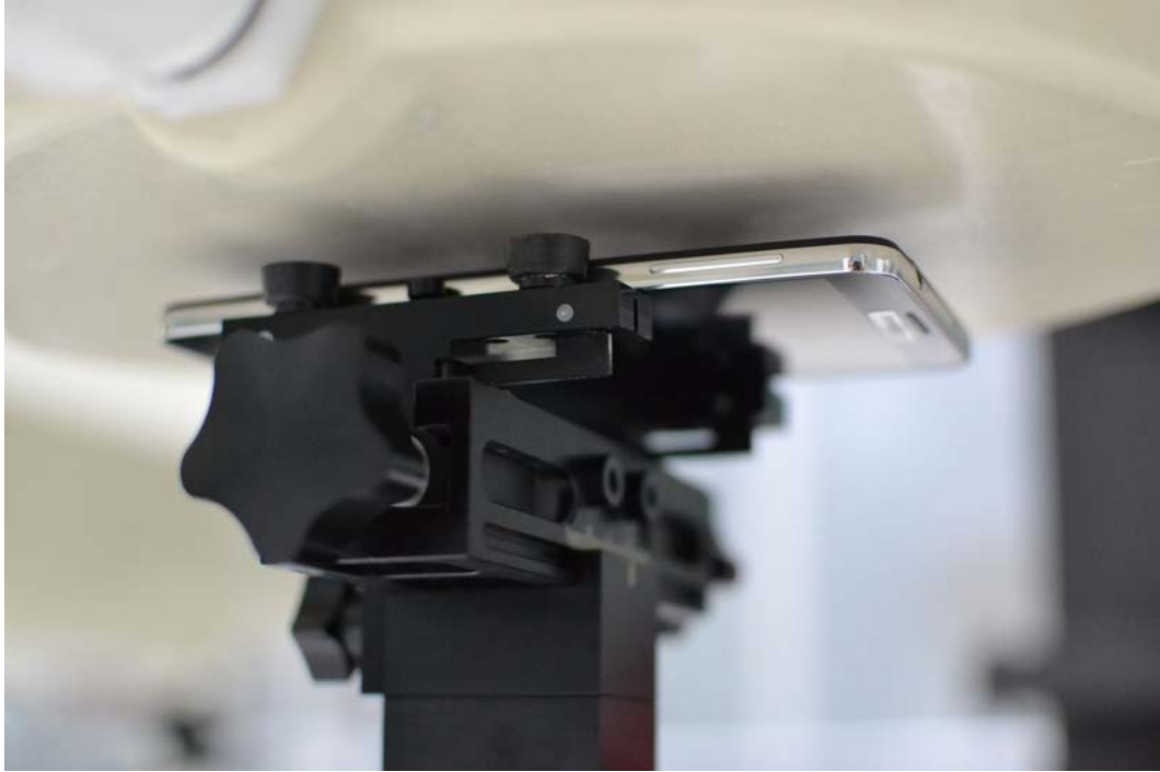
SAR Test Setup Photo 5– Back at 1.0 cm
