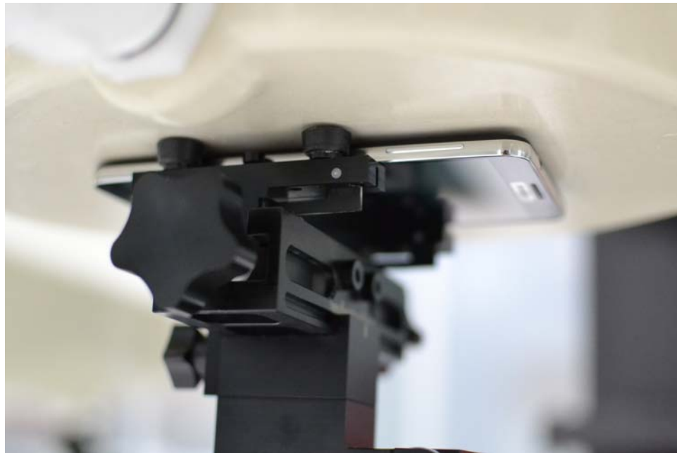
SAR Test Setup Photo 6: Back Side at 0.0 cm
