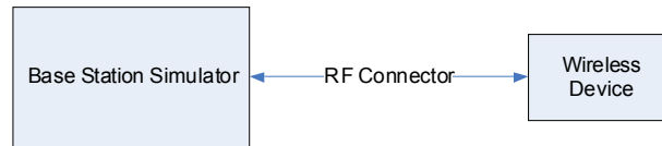
Figure 9-1 Power Measurement Setup
