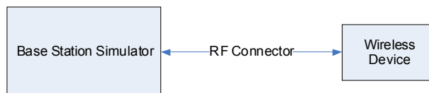
Figure 9-2 Power Measurement Setup
