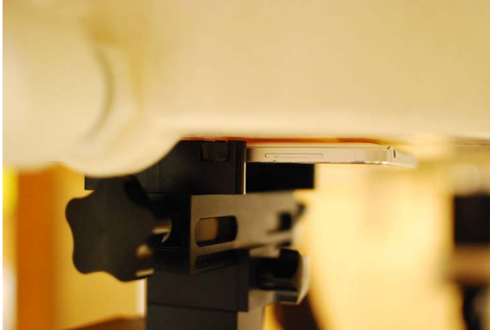
SAR Test Setup Photo 11: Back at 0.0 cm
