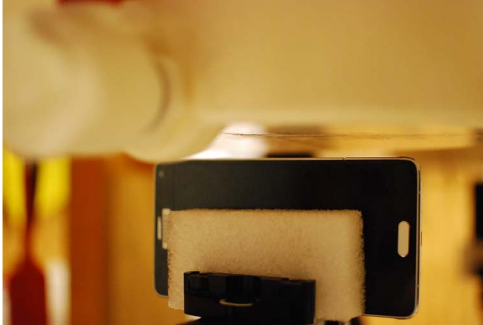
SAR Test Setup Photo 9: Right at 1.0 cm
