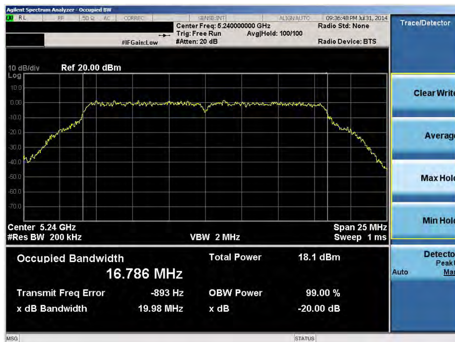
Plot 6-63. 20dB Bandwidth Plot (20MHz BW 802.11a (UNII Band 1) – Ch. 48)
