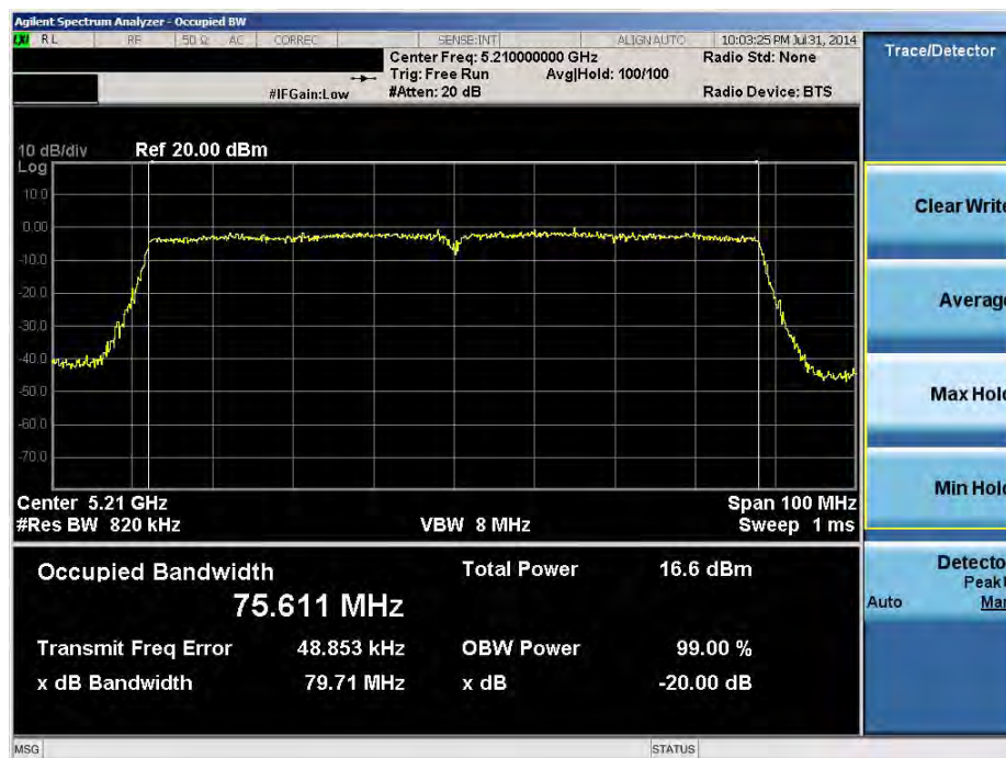
Plot 6-68. 20dB Bandwidth Plot (80MHz BW 802.11ac (UNII Band 1) – Ch. 42)
