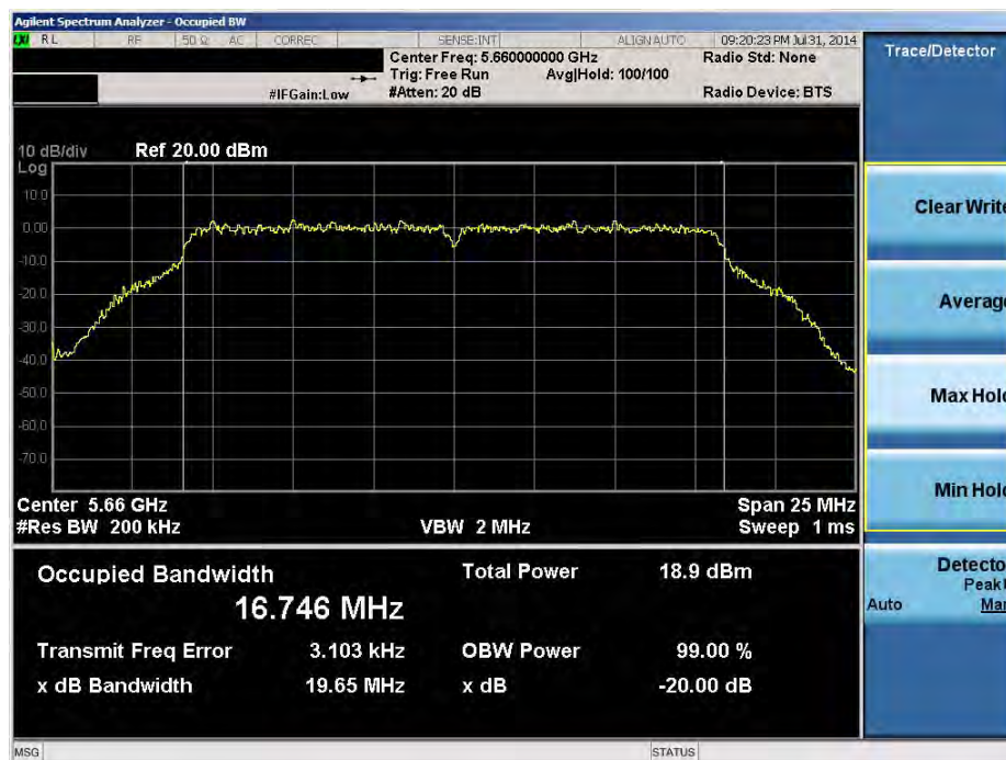
Plot 6-31. 20dB Bandwidth Plot (20MHz BW 802.11n (UNII Band 2C) – Ch. 132)
