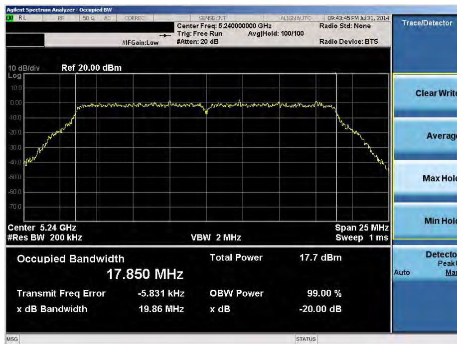
Plot 6-64. 20dB Bandwidth Plot (20MHz BW 802.11n (UNII Band 1) – Ch. 48)
