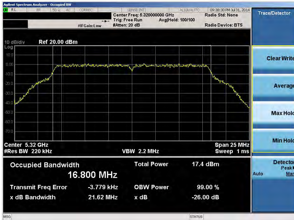
Plot 6-46. 26dB Bandwidth Plot (802.11a (UNII Band 2A) – Ch. 64)
