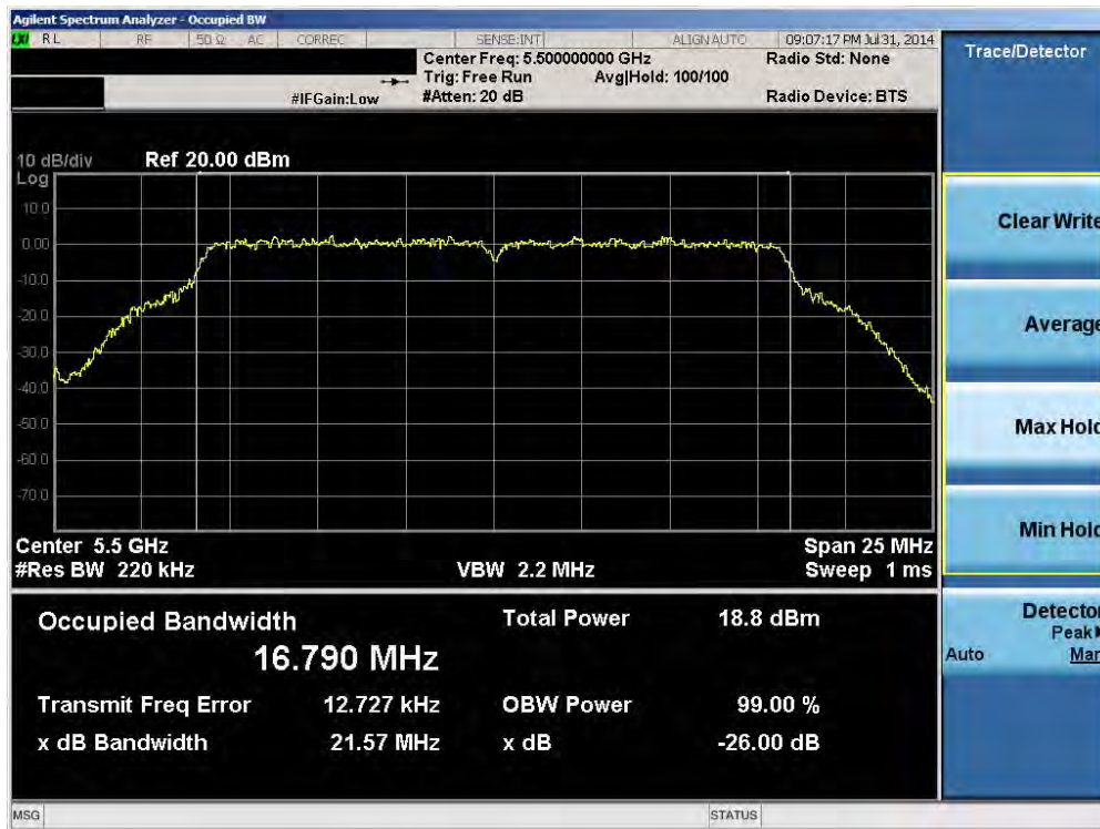
Plot 6-19. 26dB Bandwidth Plot (802.11a (UNII Band 2C) – Ch. 100)
