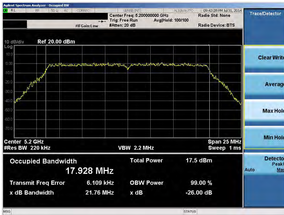
Plot 6-39. 26dB Bandwidth Plot (20MHz BW 802.11n (UNII Band 1) – Ch. 40)
