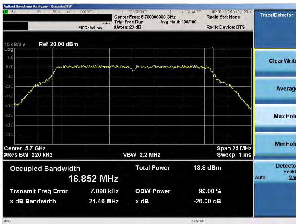
Plot 6-24. 26dB Bandwidth Plot (20MHz BW 802.11n (UNII Band 2C) – Ch. 140)
