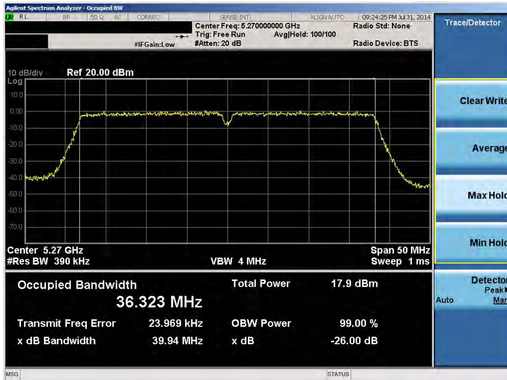
Plot 6-16. 26dB Bandwidth Plot (40MHz BW 802.11n (UNII Band 2A) – Ch. 54)
