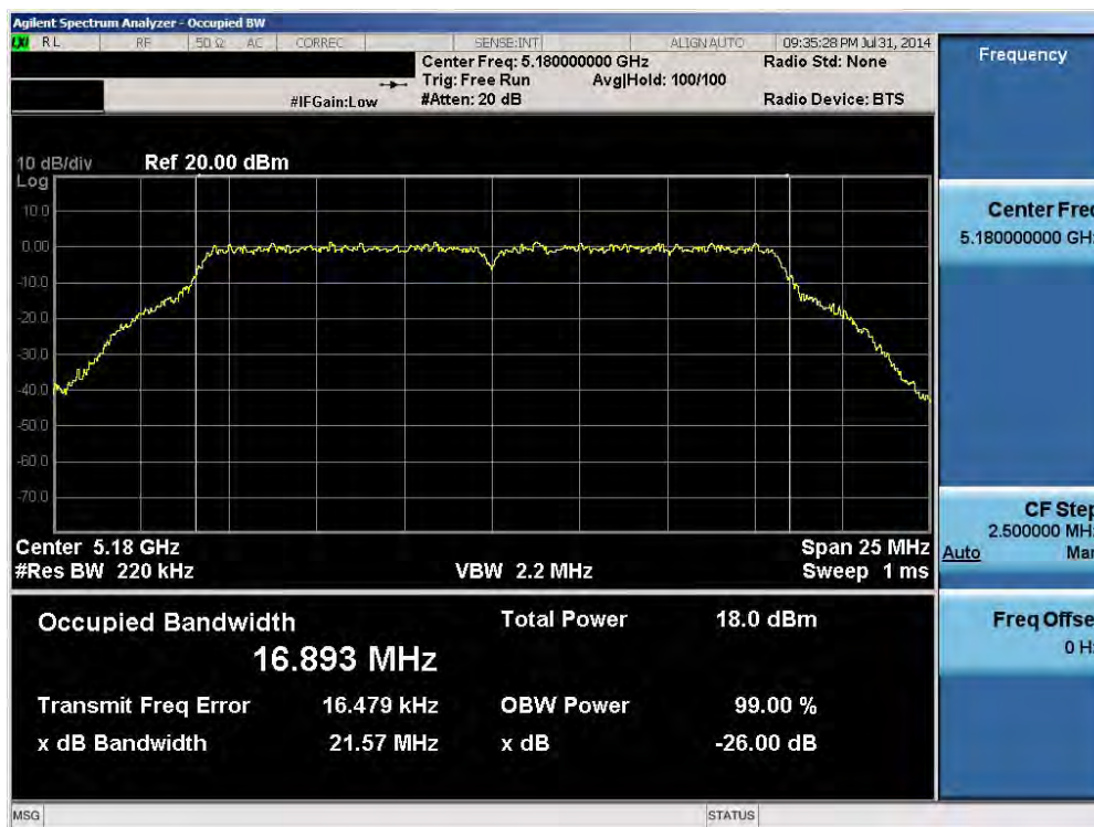
Plot 6-35. 26dB Bandwidth Plot (802.11a (UNII Band 1) – Ch. 36)
