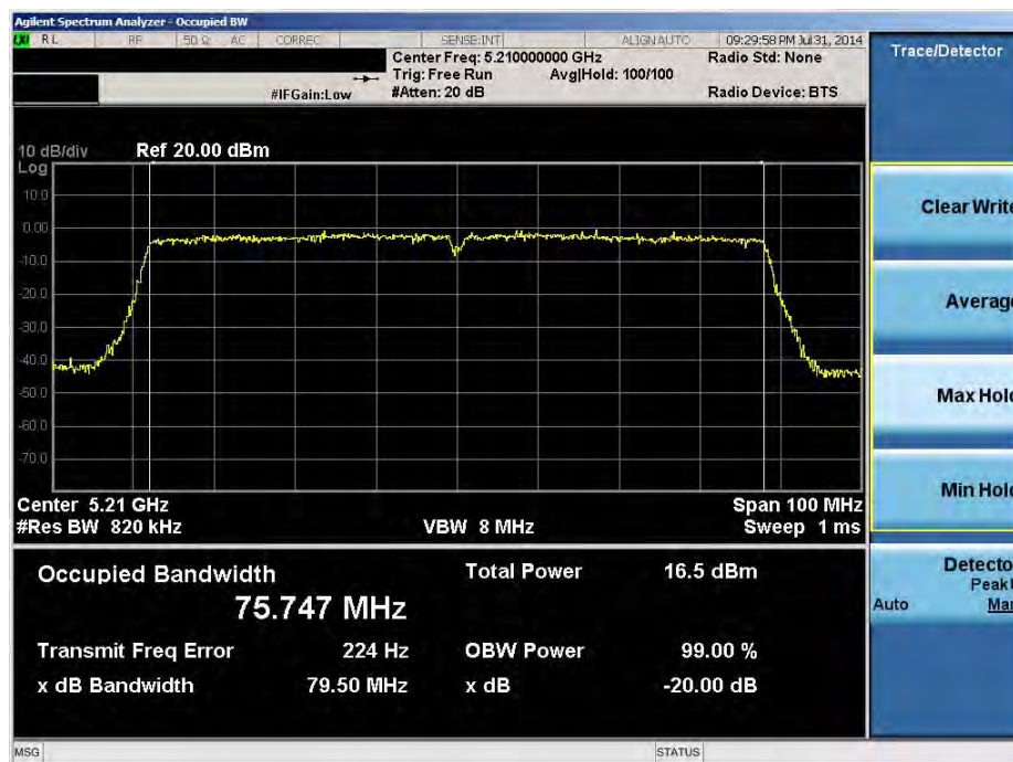
Plot 6-34. 20dB Bandwidth Plot (80MHz BW 802.11ac (UNII Band 1) – Ch. 42)
