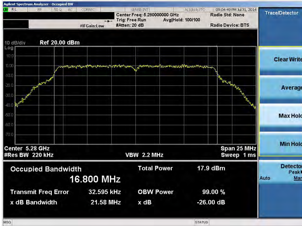
Plot 6-11. 26dB Bandwidth Plot (802.11a (UNII Band 2A) – Ch. 56)
