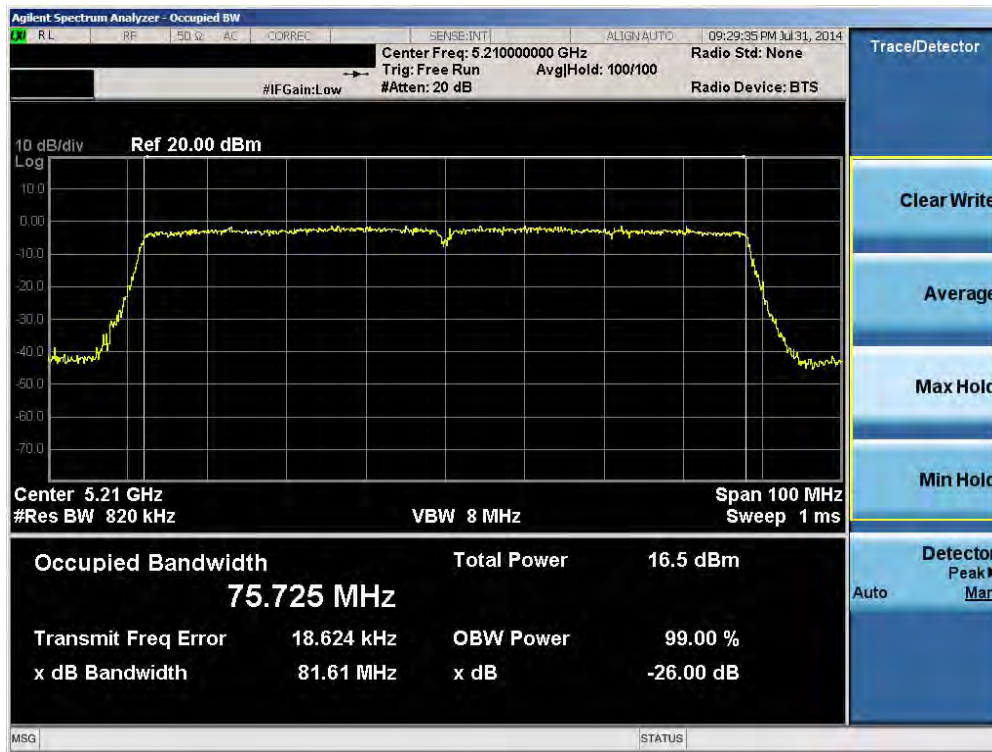
Plot 6-9. 26dB Bandwidth Plot (80MHz BW 802.11ac (UNII Band 1) – Ch. 42)
