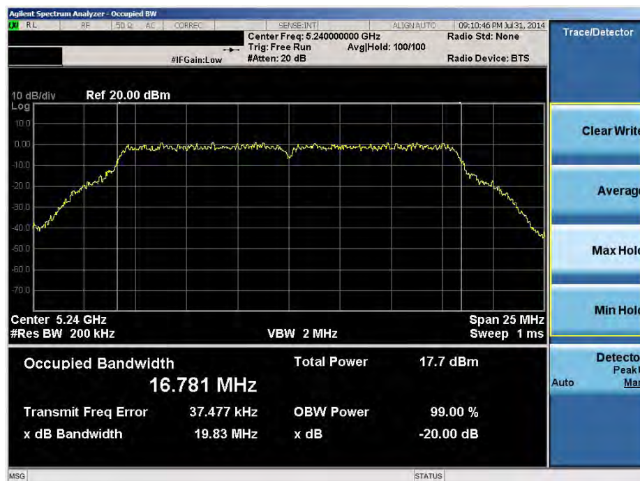
Plot 6-29. 20dB Bandwidth Plot (20MHz BW 802.11a (UNII Band 1) – Ch. 48)
