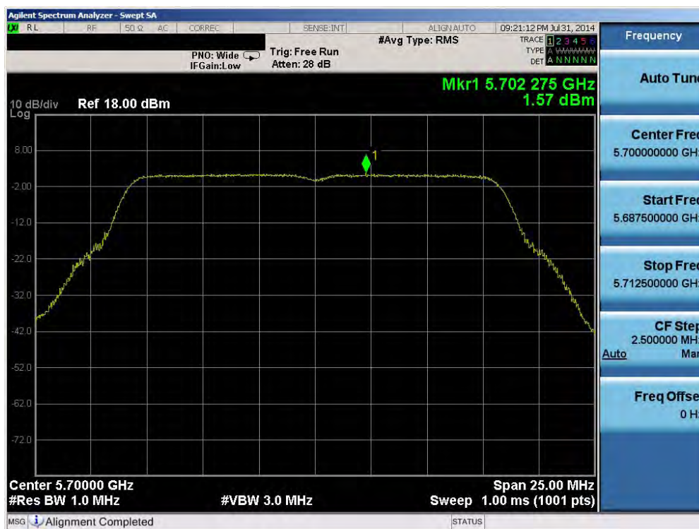
Plot 6-92. Peak Power Spectral Density Plot (20MHz BW 802.11n (UNII Band 2C) – Ch. 140)
