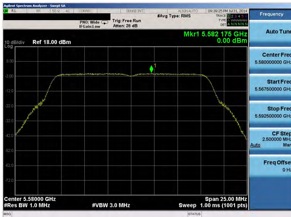
Plot 6-116. Peak Power Spectral Density Plot (802.11a (UNII Band 2C) – Ch. 116)
