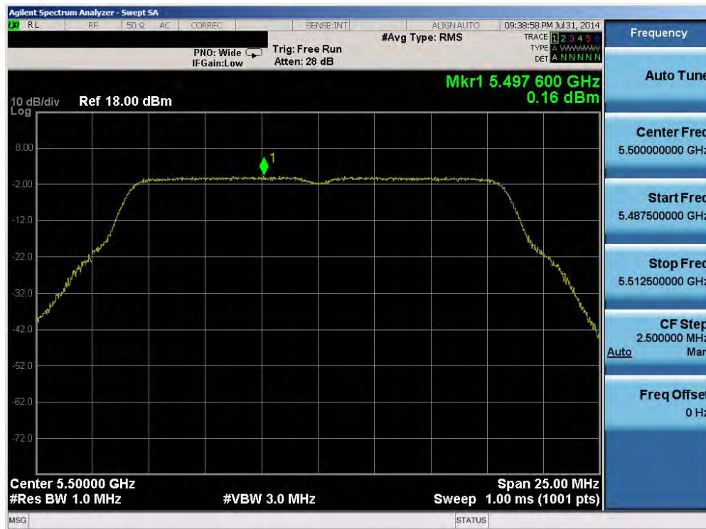
Plot 6-115. Peak Power Spectral Density Plot (802.11a (UNII Band 2C) – Ch. 100)
