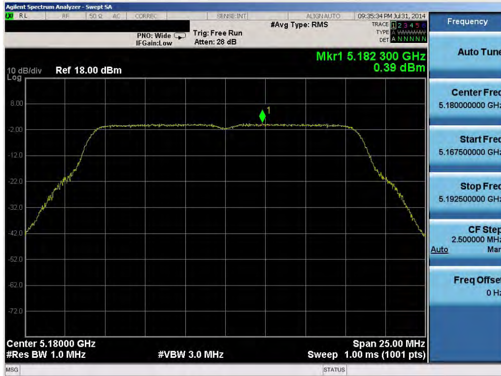
Plot 6-97. Peak Power Spectral Density Plot (802.11a (UNII Band 1) – Ch. 36)
