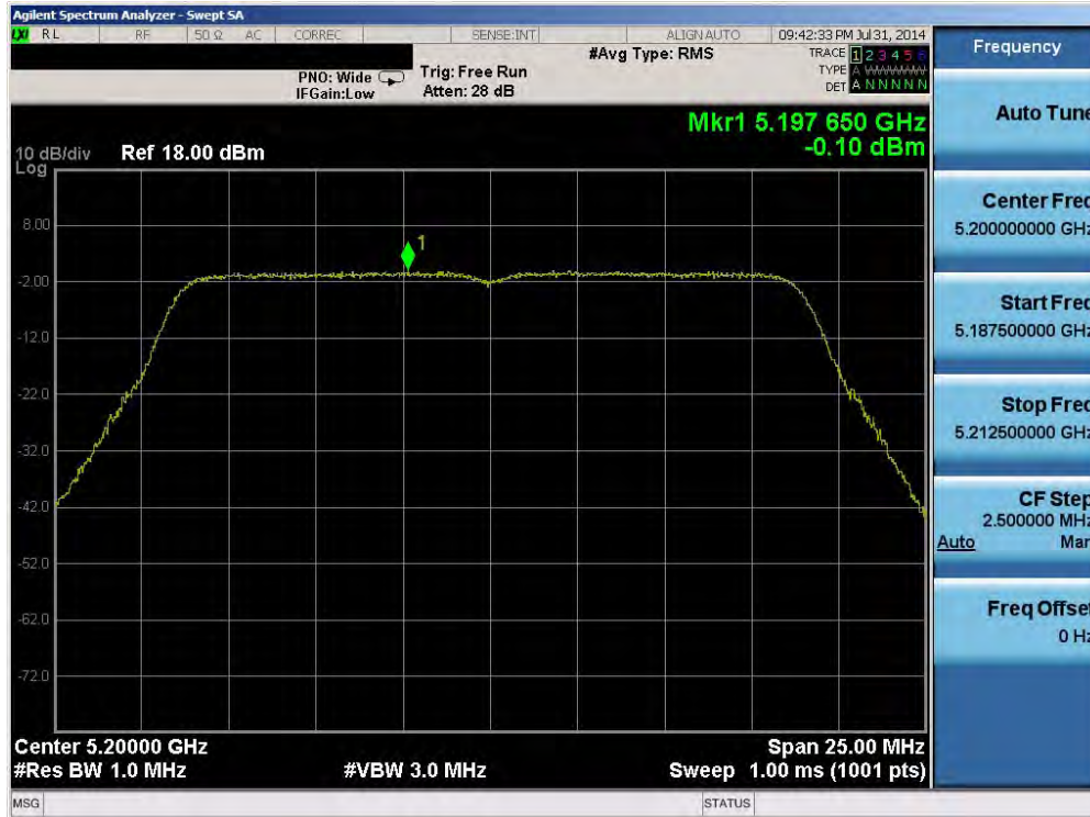
Plot 6-101. Peak Power Spectral Density Plot (20MHz BW 802.11n (UNII Band 1) – Ch. 40)
