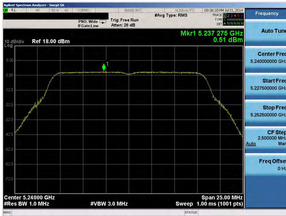
Plot 6-99. Peak Power Spectral Density Plot (802.11a (UNII Band 1) – Ch. 48)
