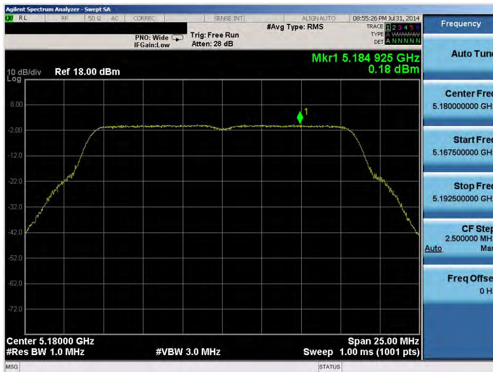
Plot 6-69. Peak Power Spectral Density Plot (802.11a (UNII Band 1) – Ch. 36)
