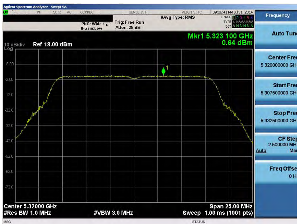
Plot 6-80. Peak Power Spectral Density Plot (802.11a (UNII Band 2A) – Ch. 64)
