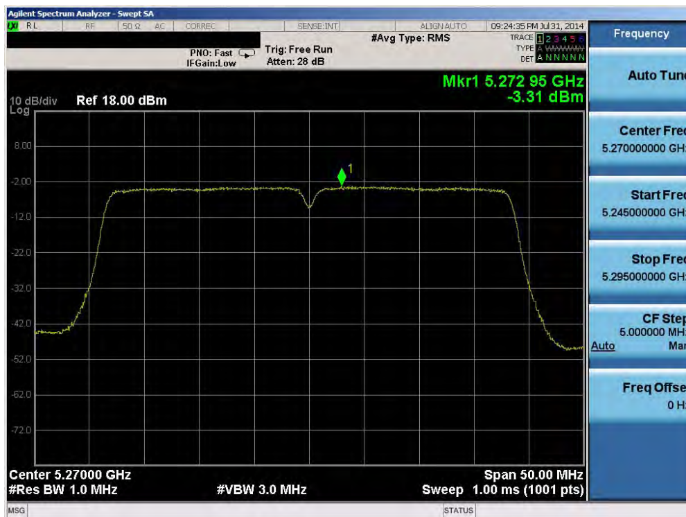
Plot 6-84. Peak Power Spectral Density Plot (40MHz BW 802.11n (UNII Band 2A) – Ch. 54)
