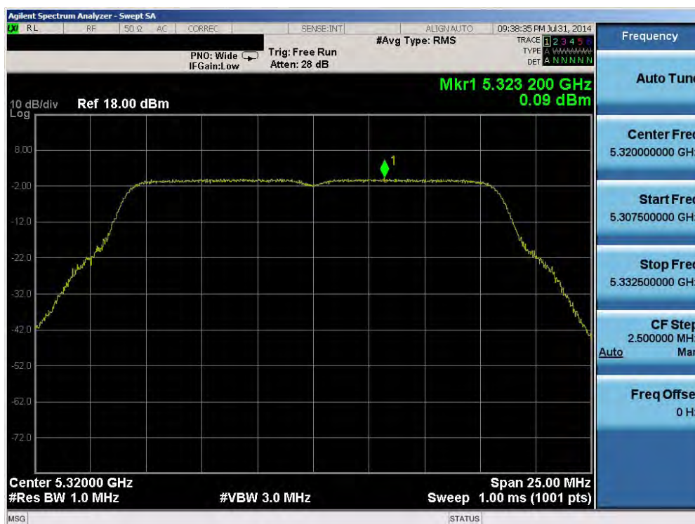
Plot 6-108. Peak Power Spectral Density Plot (802.11a (UNII Band 2A) – Ch. 64)
