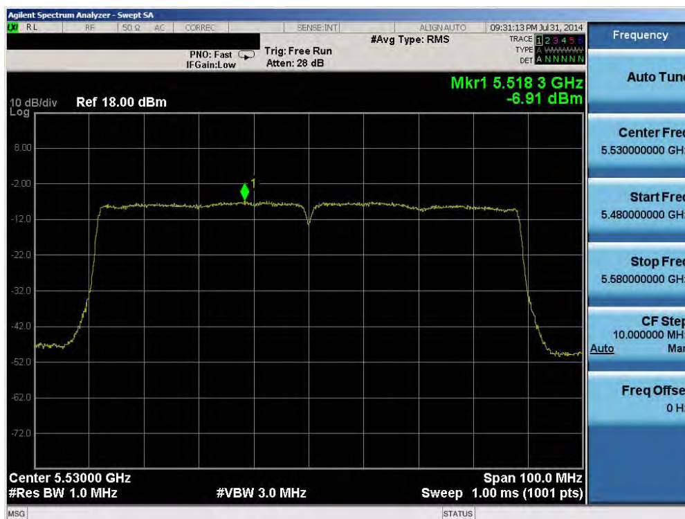
Plot 6-96. Peak Power Spectral Density Plot (80MHz BW 802.11ac (UNII Band 2C) – Ch. 106)
