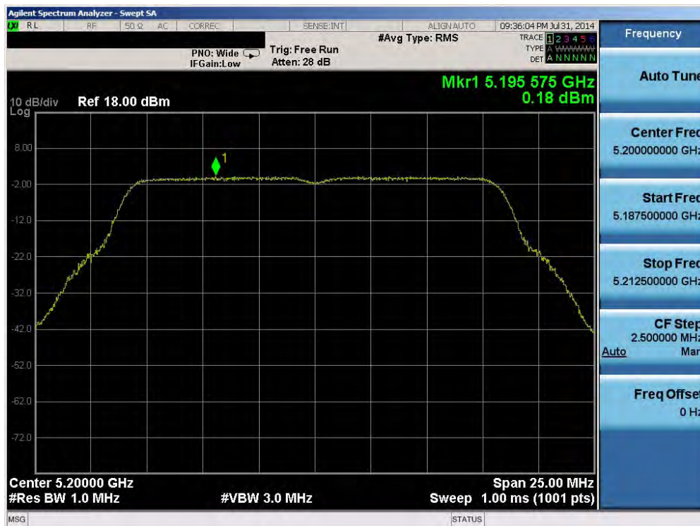
Plot 6-98. Peak Power Spectral Density Plot (802.11a (UNII Band 1) – Ch. 40)
