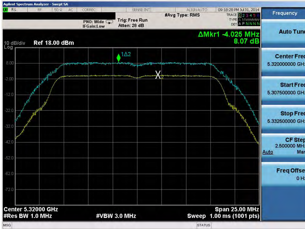
Plot 6-126. Peak Excursion Ratio Plot (20MHz BW 802.11n (UNII Band 2A) – Ch. 64)
