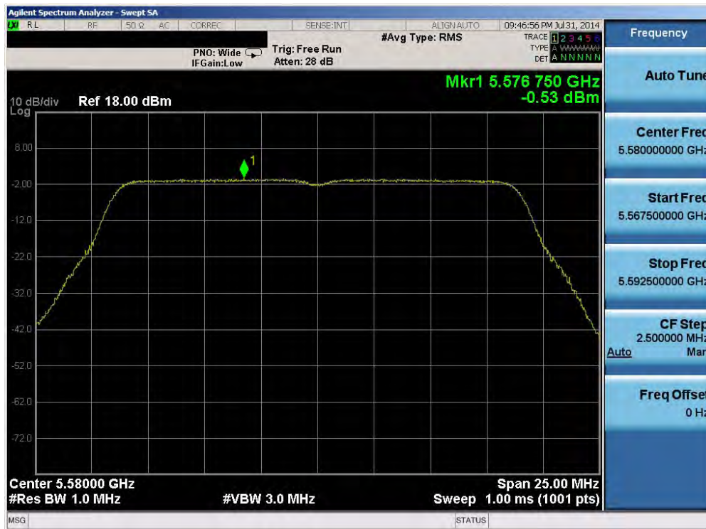
Plot 6-119. Peak Power Spectral Density Plot (20MHz BW 802.11n (UNII Band 2C) – Ch. 116)
