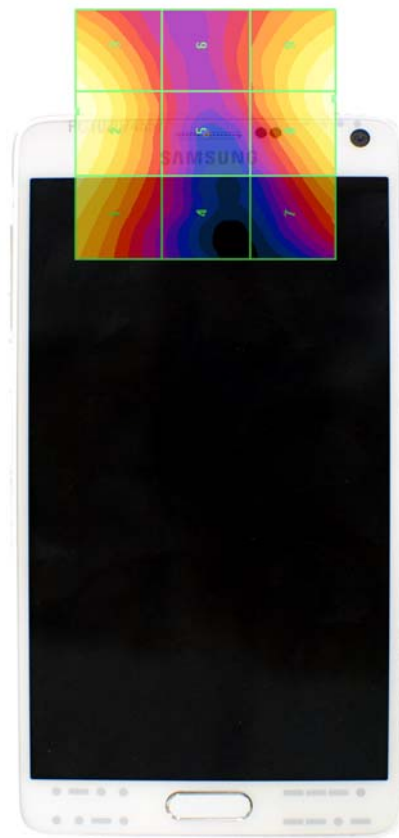
Figure 18-5 E-Field WD Scan overlay
