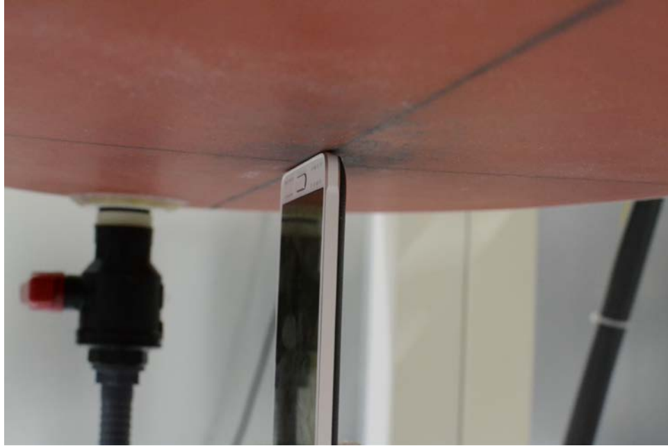
SAR Test Setup Photo 19 – Bottom Edge at 0.0 cm (Extremity), Wireless Charging Cover
