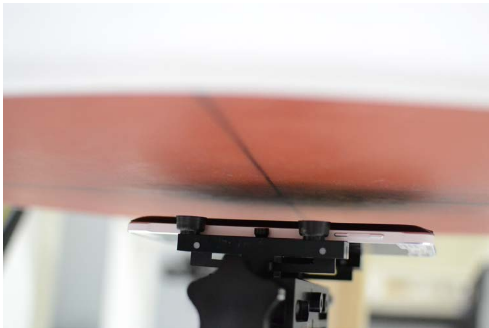
SAR Test Setup Photo 12 - Back Side at 1.5 cm (Body-worn), Wireless Charging Cover
