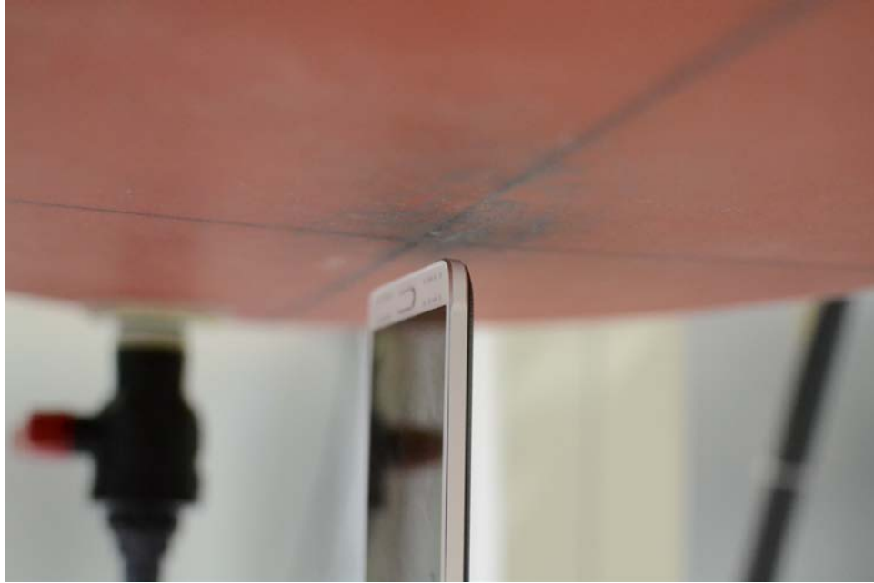
SAR Test Setup Photo 21 – Bottom Edge at 1.0 cm (Hotspot), Wireless Charging Cover
