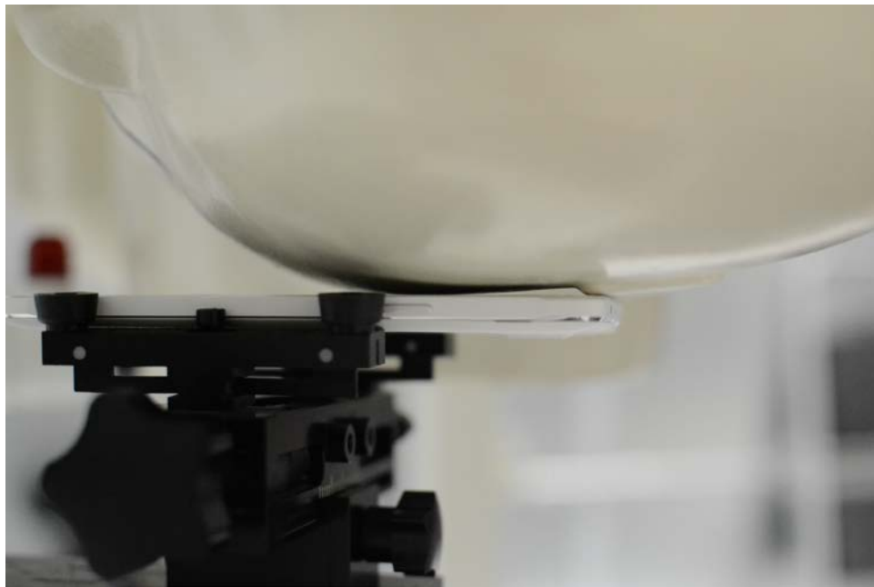
SAR Test Setup Photo 4 – Left Cheek, Standard Cover
