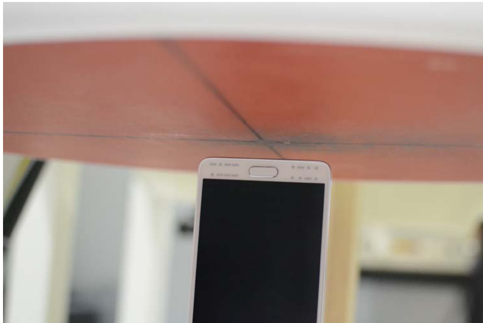
SAR Test Setup Photo 20 – Bottom Edge at 1.0 cm (Hotspot), Standard Cover
