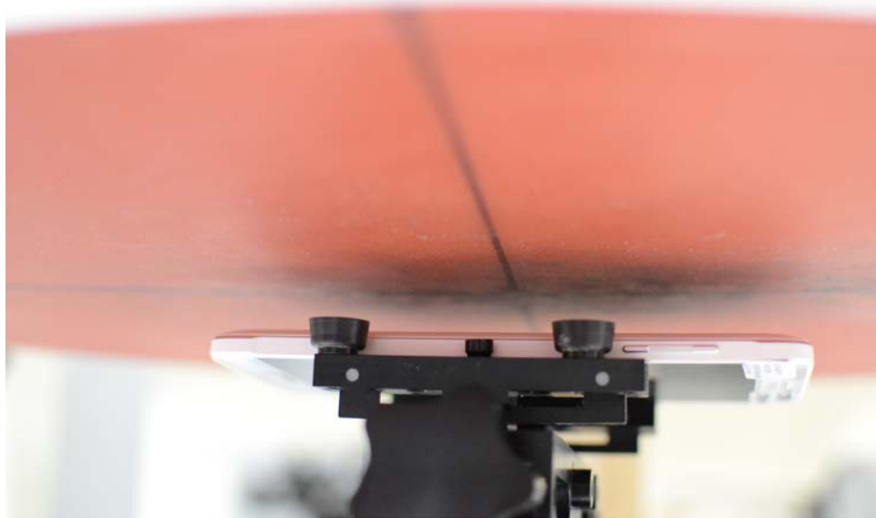
SAR Test Setup Photo 11 – Back Side at 1.5 cm (Body-worn), Standard Cover
