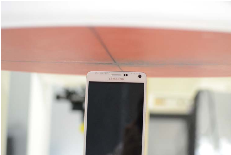
SAR Test Setup Photo 17 – Top Edge at 1.0 cm (Hotspot), Standard Cover
