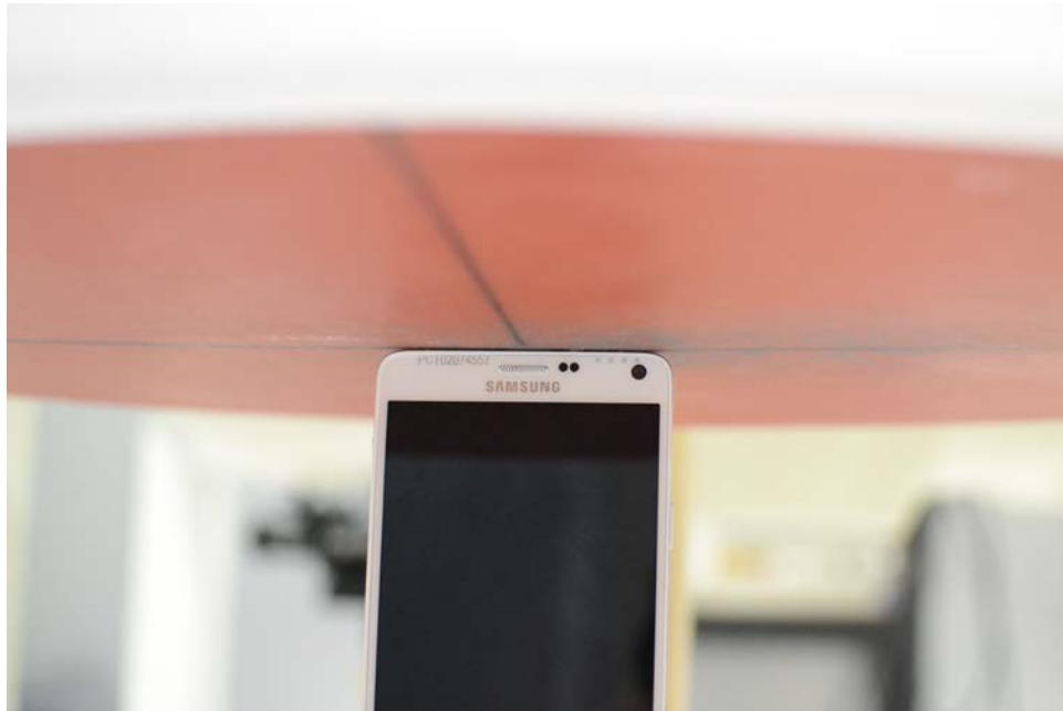
SAR Test Setup Photo 16 – Top Edge at 0.0 cm (Extremity), Standard Cover
