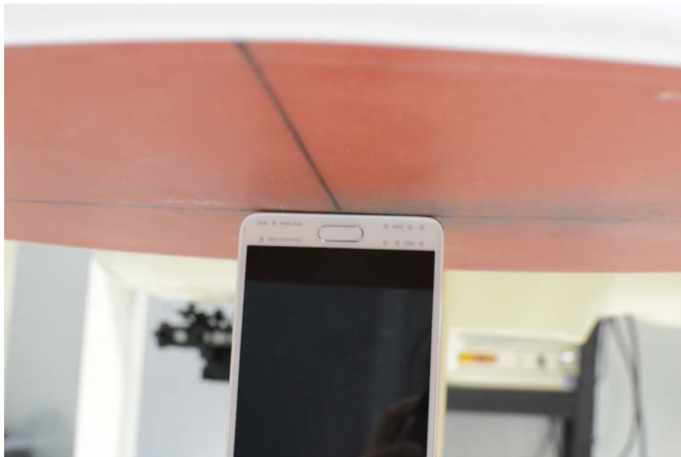
SAR Test Setup Photo 18 – Bottom Edge at 0.0 cm (Extremity), Standard Cover
