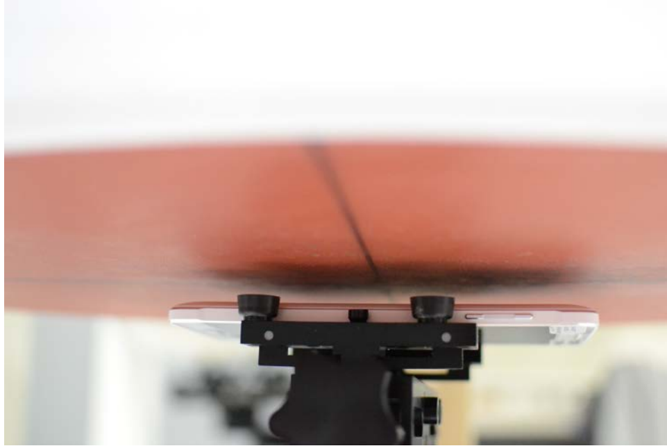
SAR Test Setup Photo 9 – Back Side at 1.0 cm (Hotspot), Standard Cover
