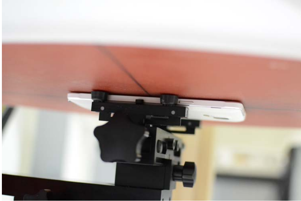
SAR Test Setup Photo 13— Front Side at 0.0 cm (Extremity), Standard Cover
