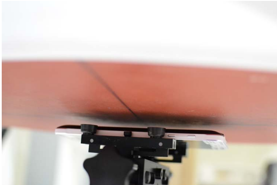
SAR Test Setup Photo 10 – Back Side at 1.0 cm (Hotspot), Wireless Charging Cover
