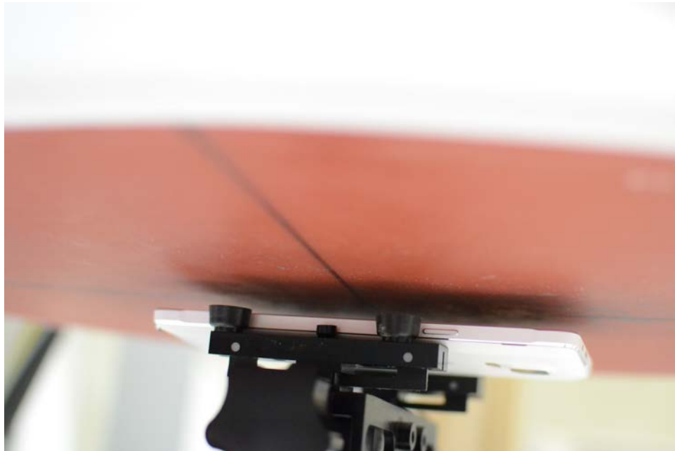
SAR Test Setup Photo 14 - Front Side at 1.0 cm (Hotspot), Standard Cover
