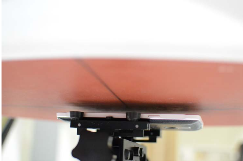
SAR Test Setup Photo 15 - Front Side at 1.0 cm (Hotspot), Wireless Charging Cover
