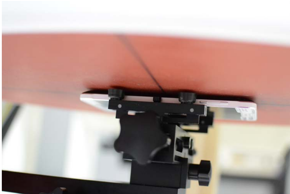
SAR Test Setup Photo 8 – Back Side at 0.0 cm (Extremity), Wireless Charging Cover
