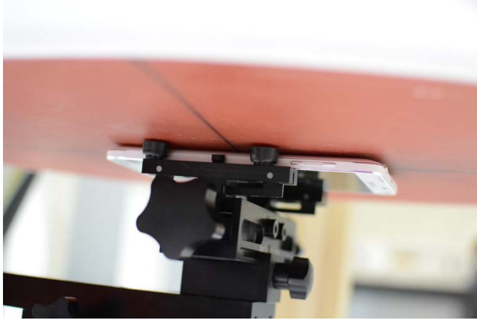
SAR Test Setup Photo 7 – Back Side at 0.0 cm (Extremity), Standard Cover
