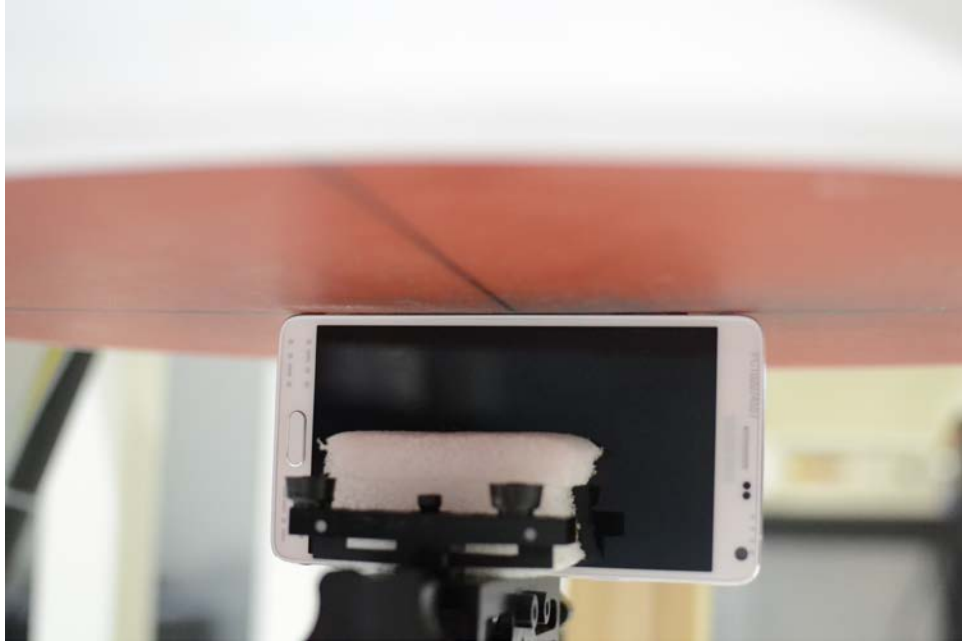
SAR Test Setup Photo 23 – Left Edge at 0.0 cm (Extremity), Standard Cover
