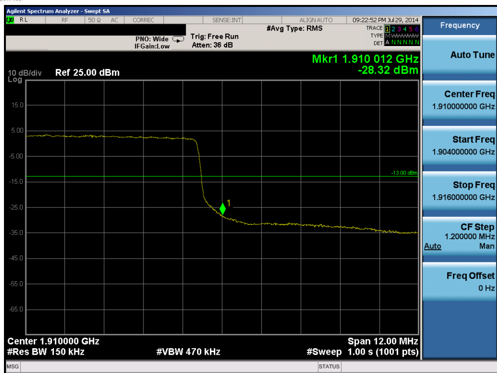
Plot 6-123. Upper Band Edge Plot (Band 2 – 15.0MHz QPSK – RB Size 75)
