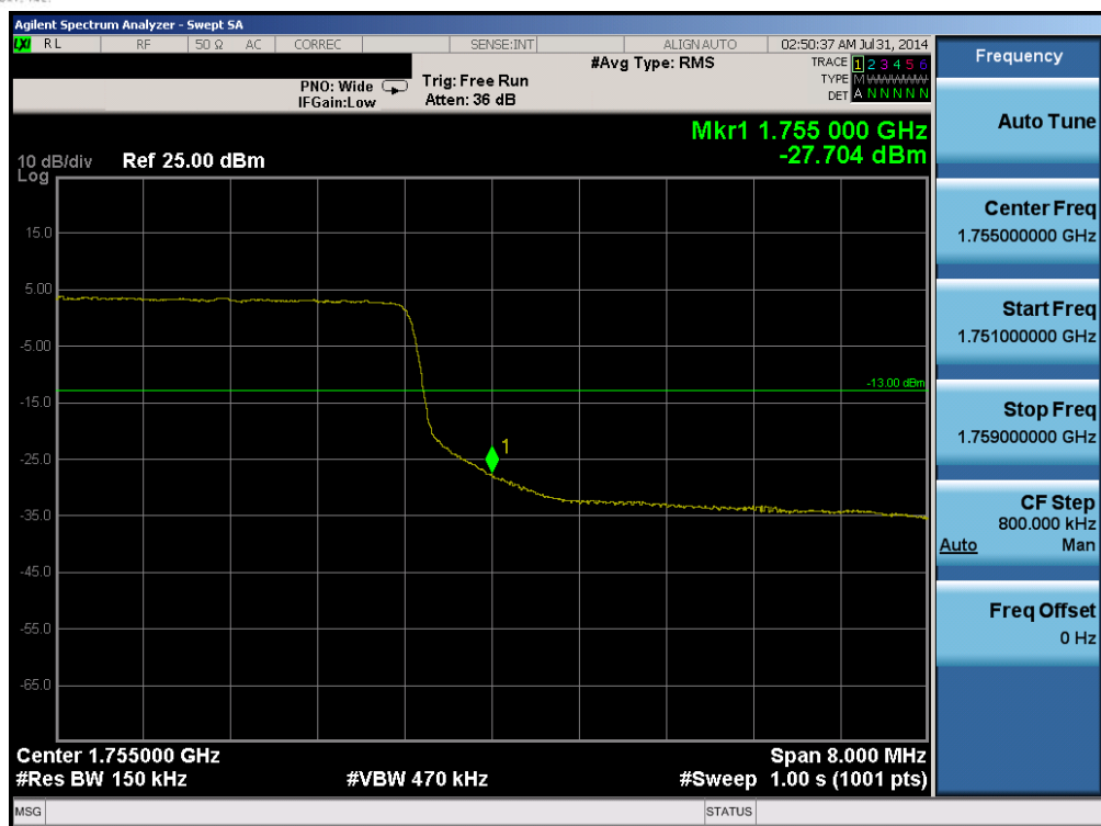
Plot 6-99. Upper Band Edge Plot (Band 4 – 15.0MHz QPSK – RB Size 75)
