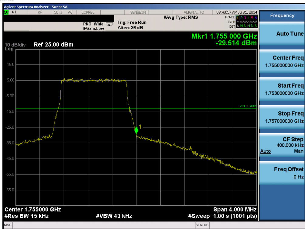
Plot 6-83. Upper Band Edge Plot (Band 4 – 1.4MHz QPSK – RB Size 6)
