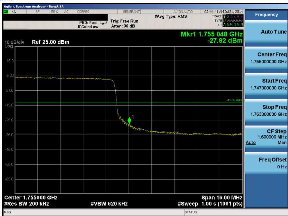
Plot 6-103. Upper Band Edge Plot (Band 4 – 20.0MHz QPSK – RB Size 100)
