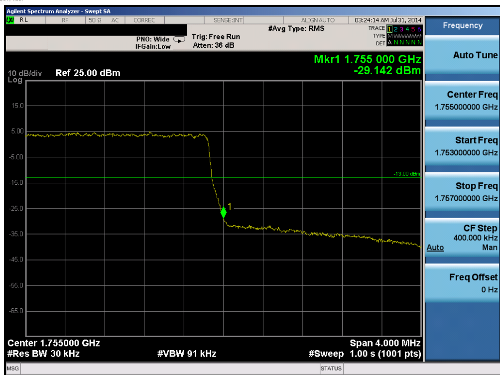
Plot 6-87. Upper Band Edge Plot (Band 4 – 3.0MHz QPSK – RB Size 15)
