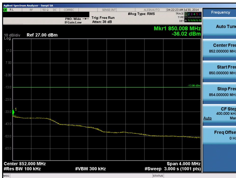
Plot 6-70. Upper Extended Band Edge Plot (Band 5 – 1.4MHz QPSK – RB Size 6)
