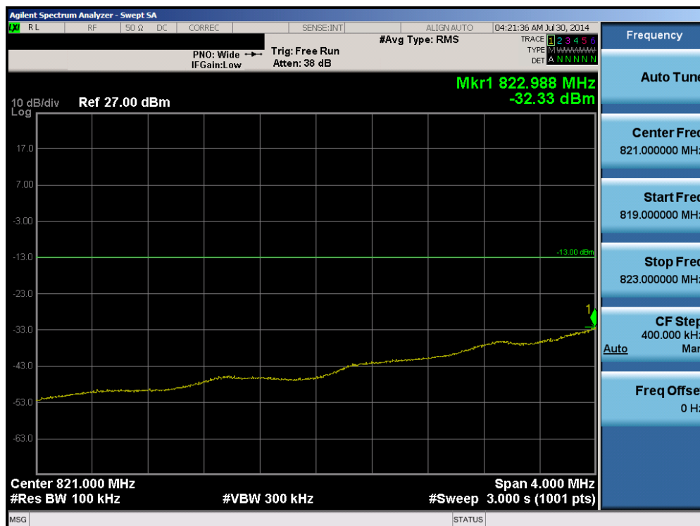
Plot 6-68. Lower Extended Band Edge Plot (Band 5 – 1.4MHz QPSK – RB Size 6)
