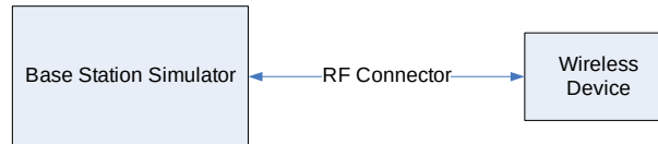
Figure 9-3 Power Measurement Setup
