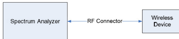
Figure 6-1. Test Instrument & Measurement Setup
