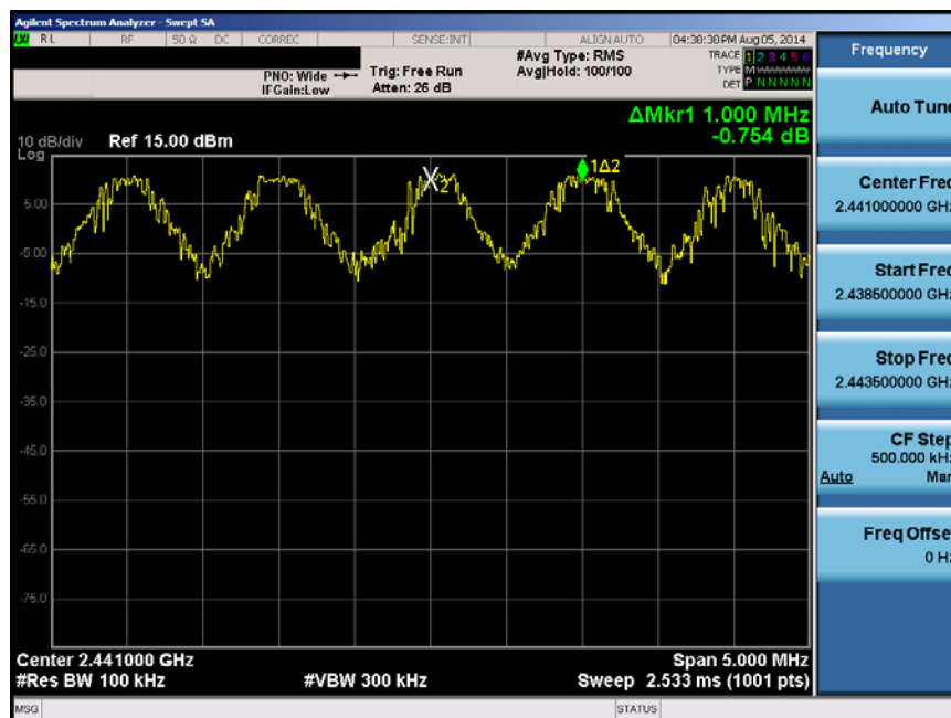
Plot 6-32. Channel Spacing Plot (Bluetooth)
