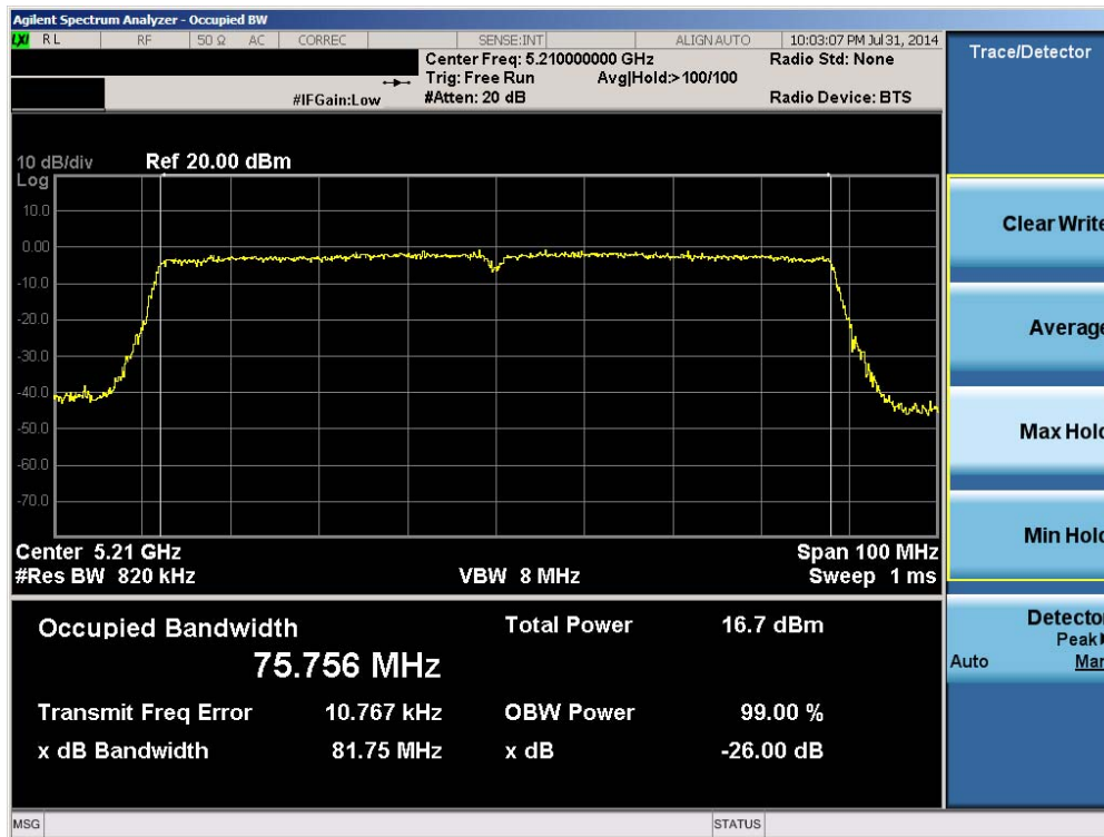
Plot 6-43. 26dB Bandwidth Plot (80MHz BW 802.11ac (UNII Band 1) – Ch. 42)
