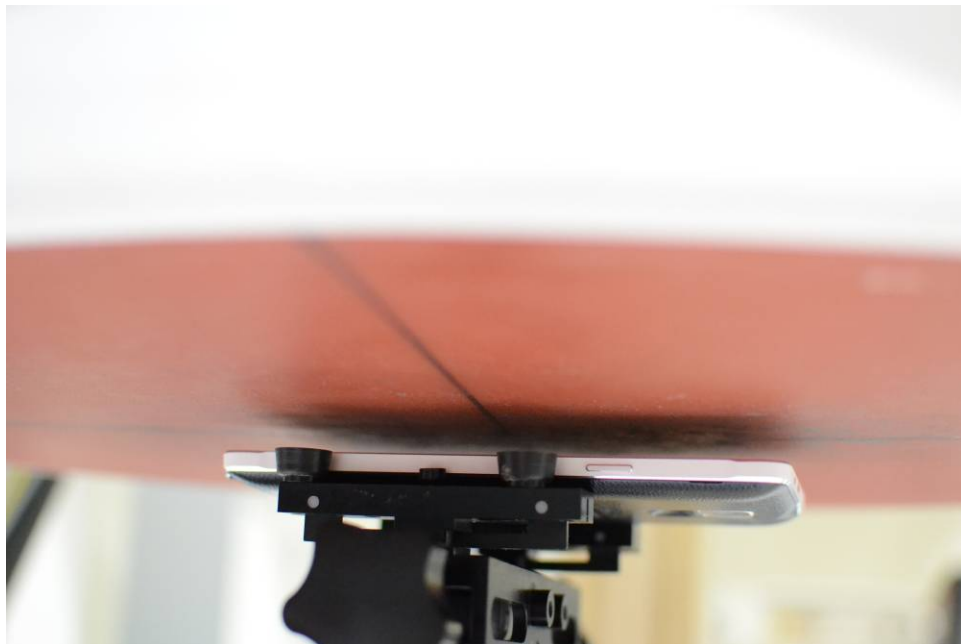
SAR Test Setup Photo 14: Front Side at 10mm, Wireless Charging Cover
