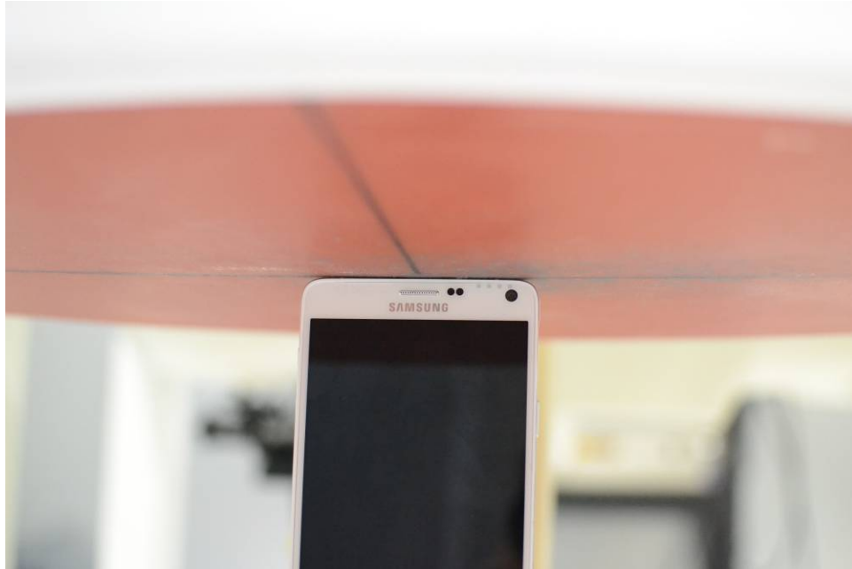
SAR Test Setup Photo 17: Top Edge at 0mm, Standard Back Cover
