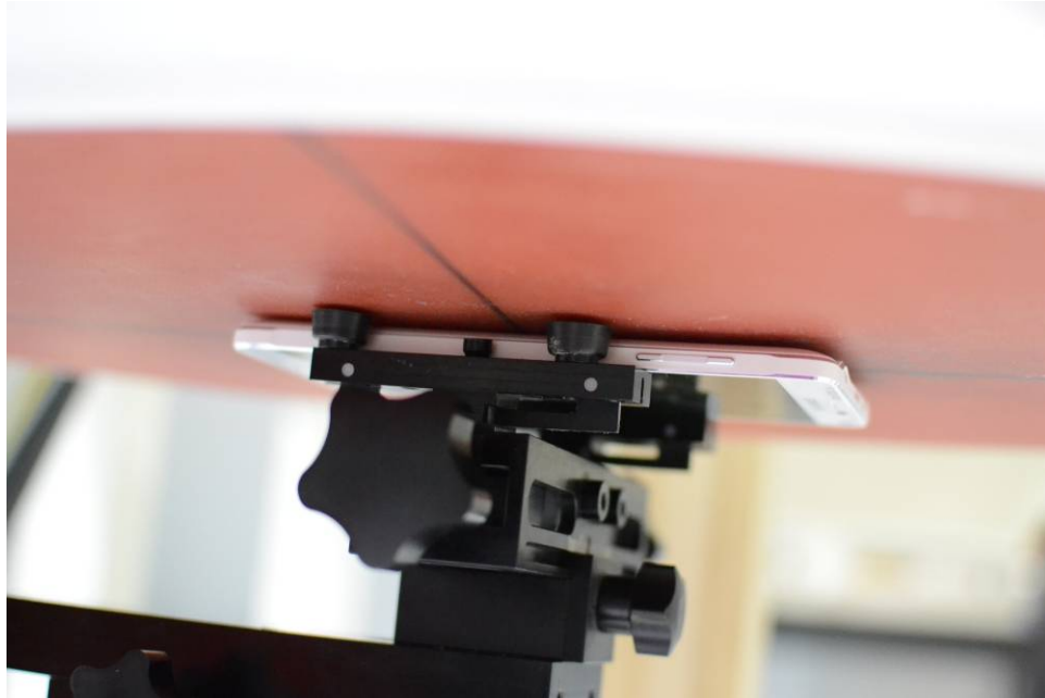
SAR Test Setup Photo 11: Back Side at 0mm, Standard Back Cover
