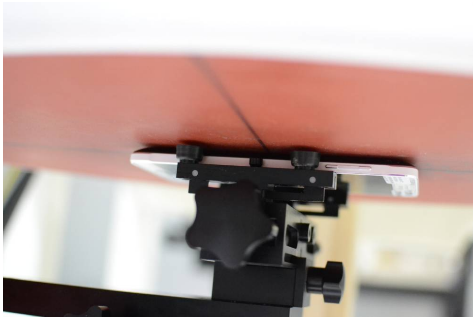
SAR Test Setup Photo 12: Back Side at 0mm, Wireless Charging Cover
