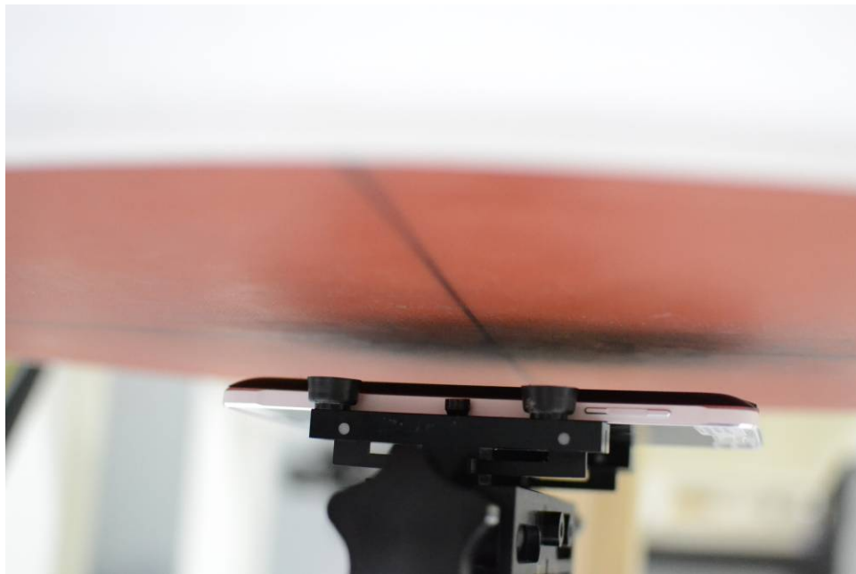
SAR Test Setup Photo 8: Back Side at 15mm, Wireless Charging Cover
