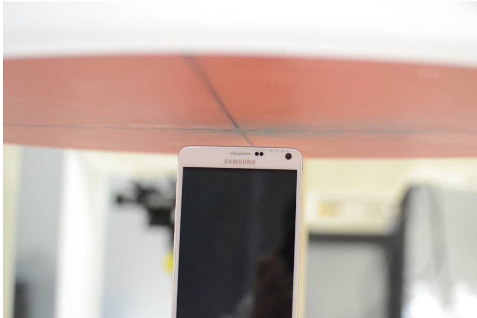
SAR Test Setup Photo 16: Top Edge at 10mm, Standard Back Cover
