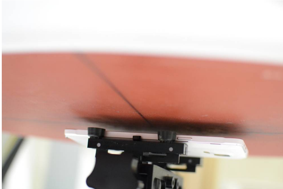
SAR Test Setup Photo 13: Front Side at 10mm, Standard Back Cover
