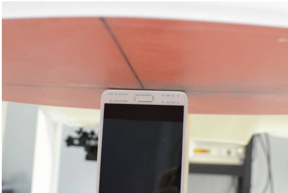
SAR Test Setup Photo 20 – Bottom Edge at 0.0 cm, Standard Cover
