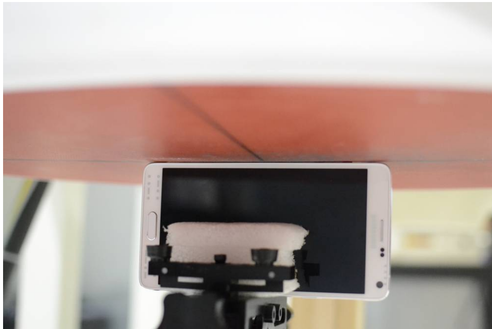
SAR Test Setup Photo 24: Left Edge at 0mm, Standard Back Cover
