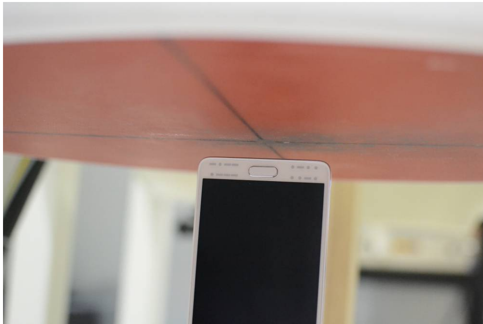
SAR Test Setup Photo 18: Bottom Edge at 10mm, Standard Back Cover
