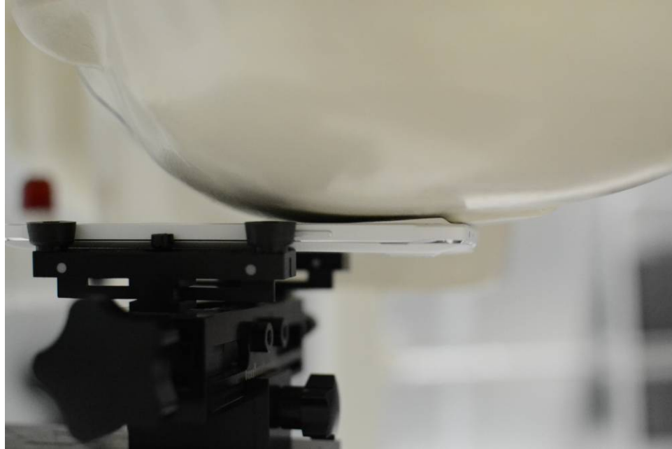
SAR Test Setup Photo 3: Left Cheek, Standard Back Cover
