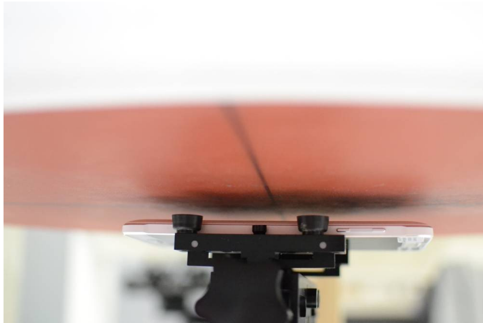
SAR Test Setup Photo 6: Back Side at 10mm, Standard Back Cover
