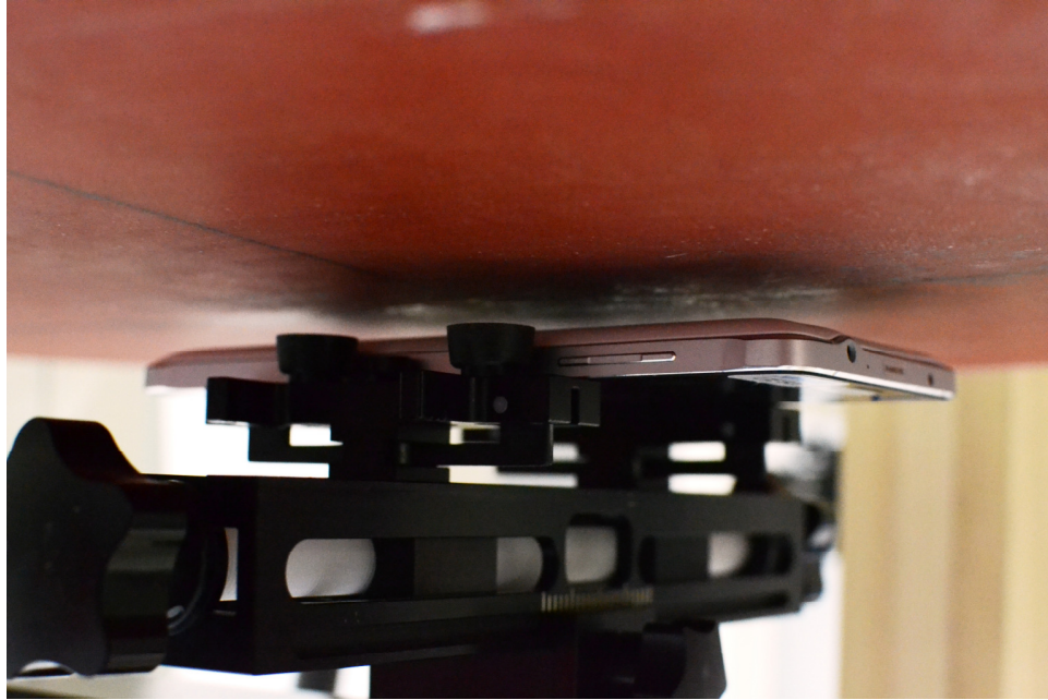
SAR Test Setup Photo 7: Back Side at 10mm, Wireless Charging Cover
