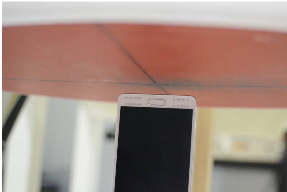
SAR Test Setup Photo 10: Bottom Edge at 10mm, Standard Back Cover
