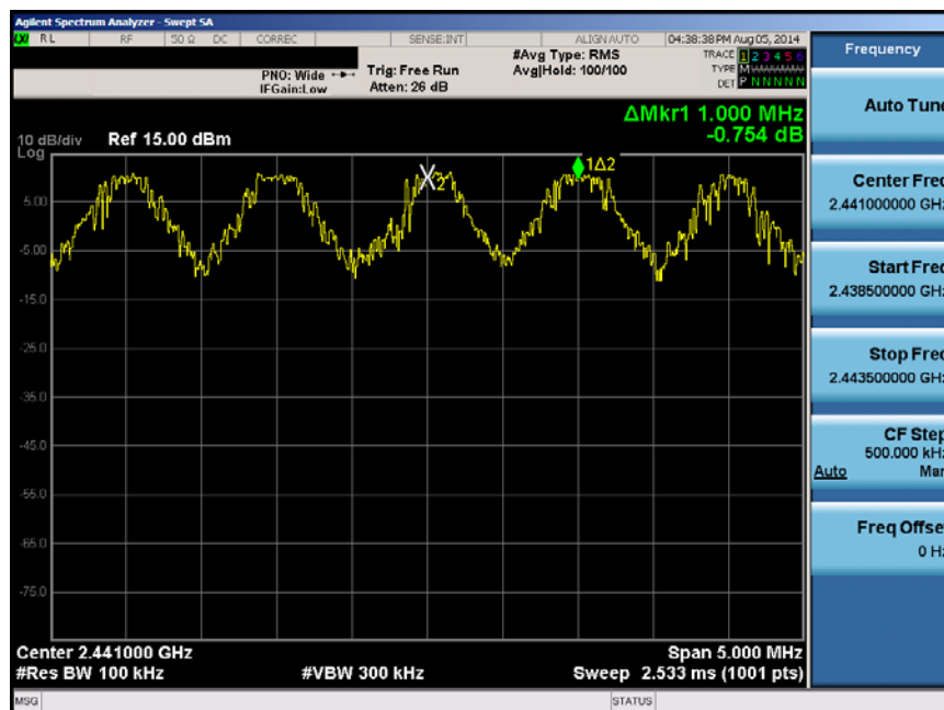
Plot 6-32. Channel Spacing Plot (Bluetooth)
