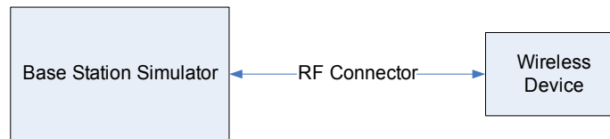
Figure 9-2 Power Measurement Setup
