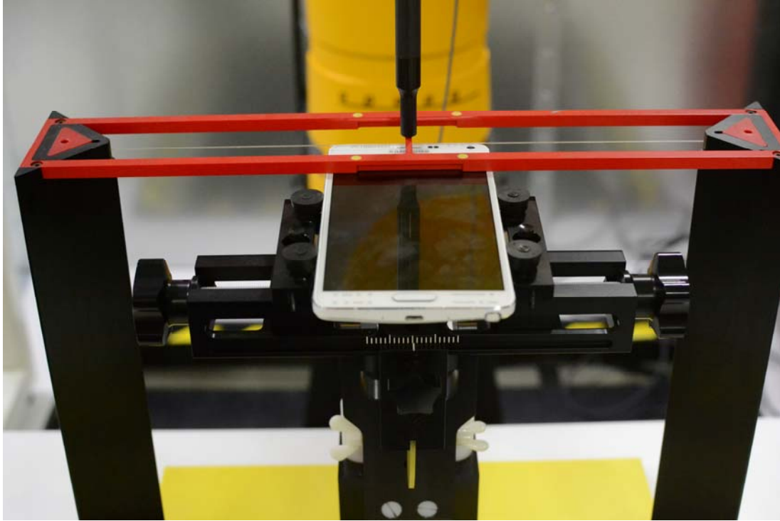
Figure 18-1 Ear Reference Point HAC Phantom Alignment
