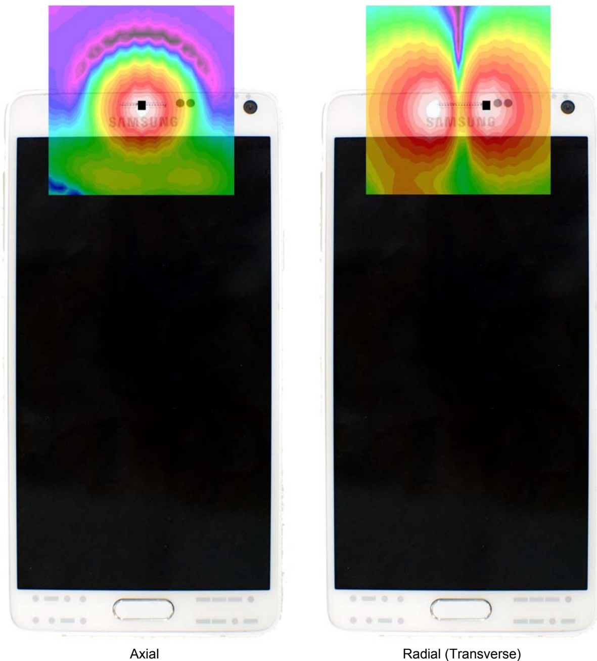
Figure 13-3 T-Coil Scan Overlay Magnetic Field Distributions
