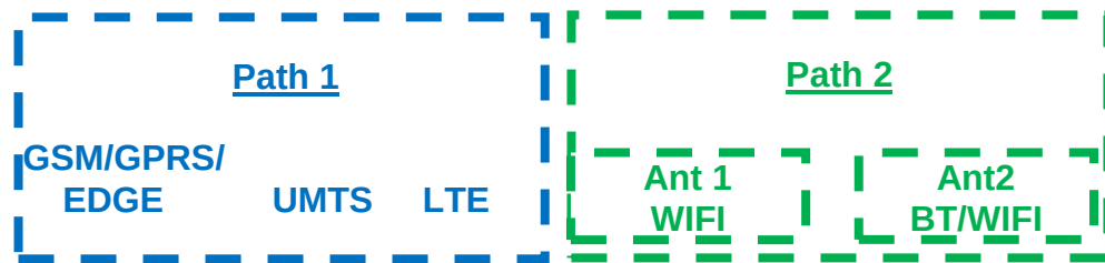
Figure 1-3 Simultaneous Transmission Paths
