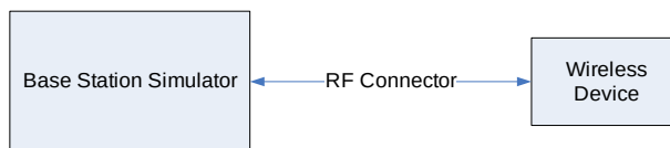
Figure 9-2 Power Measurement Setup
