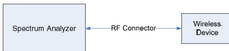
Figure 6-1. Test Instrument & Measurement Setup
