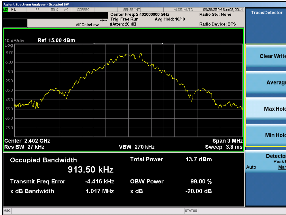
Plot 6-1. 20dB Bandwidth Plot (Bluetooth, 1Mbps – Ch. 0)
