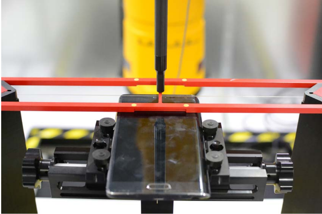
Figure 18-1 Ear Reference Point HAC Phantom Alignment
