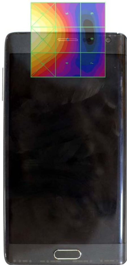
Figure 18-4 E-Field WD Scan overlay
