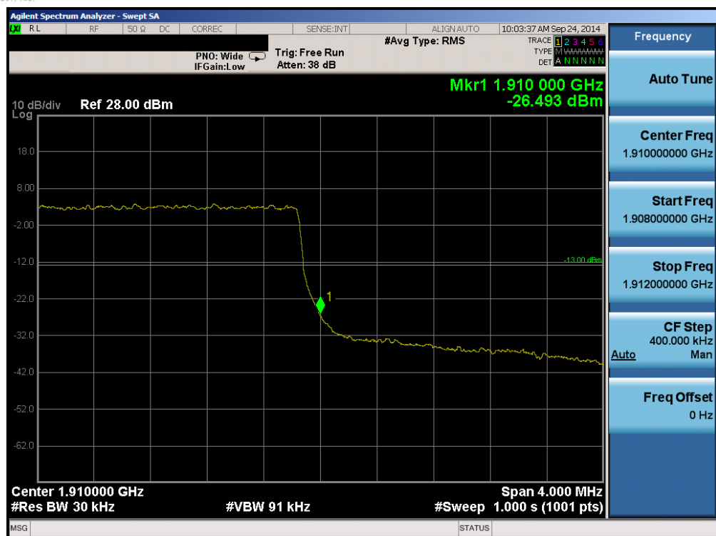
Plot 6-89. Upper Band Edge Plot (Band 2 – 3.0MHz QPSK – RB Size 15)
