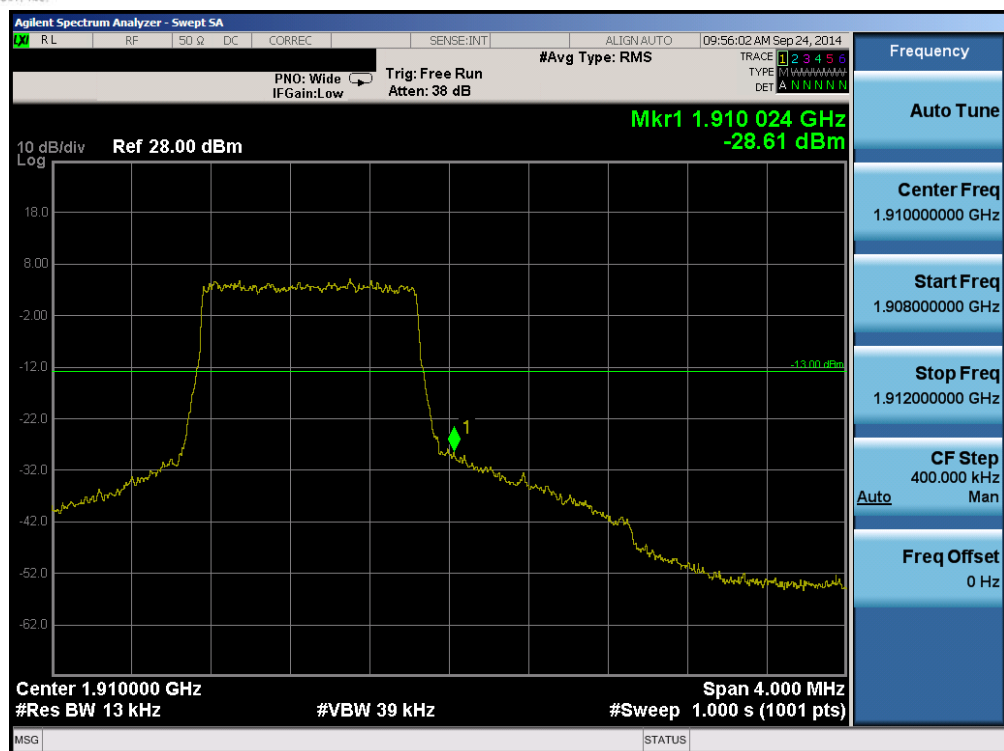
Plot 6-85. Upper Band Edge Plot (Band 2 – 1.4MHz QPSK – RB Size 6)
