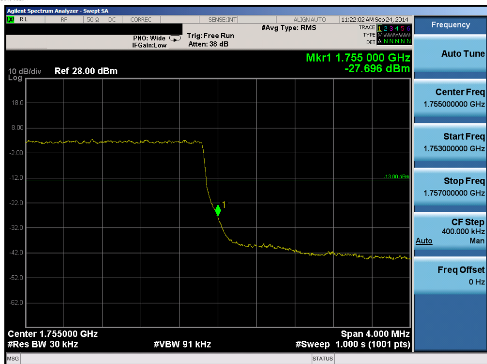
Plot 6-65. Upper Band Edge Plot (Band 4 – 3.0MHz QPSK – RB Size 15)
