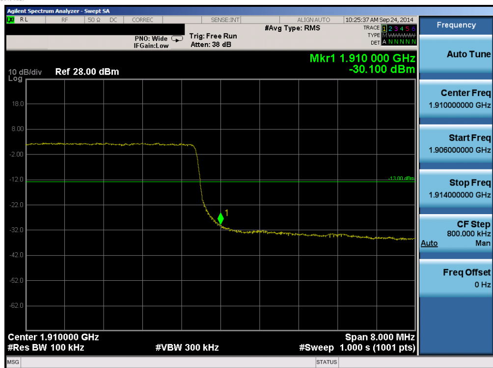
Plot 6-97. Upper Band Edge Plot (Band 2 – 10.0MHz QPSK – RB Size 50)
