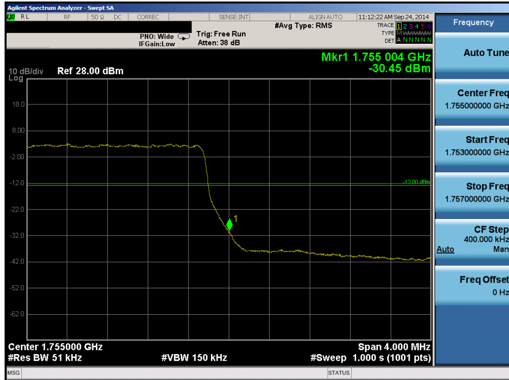
Plot 6-69. Upper Band Edge Plot (Band 4 – 5.0MHz QPSK – RB Size 25)
