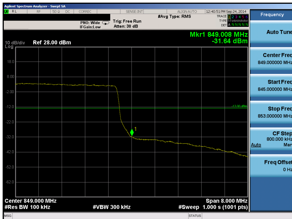
Plot 6-58. Upper Band Edge Plot (Band 5 - 10.0MHz QPSK - RB Size 50)
