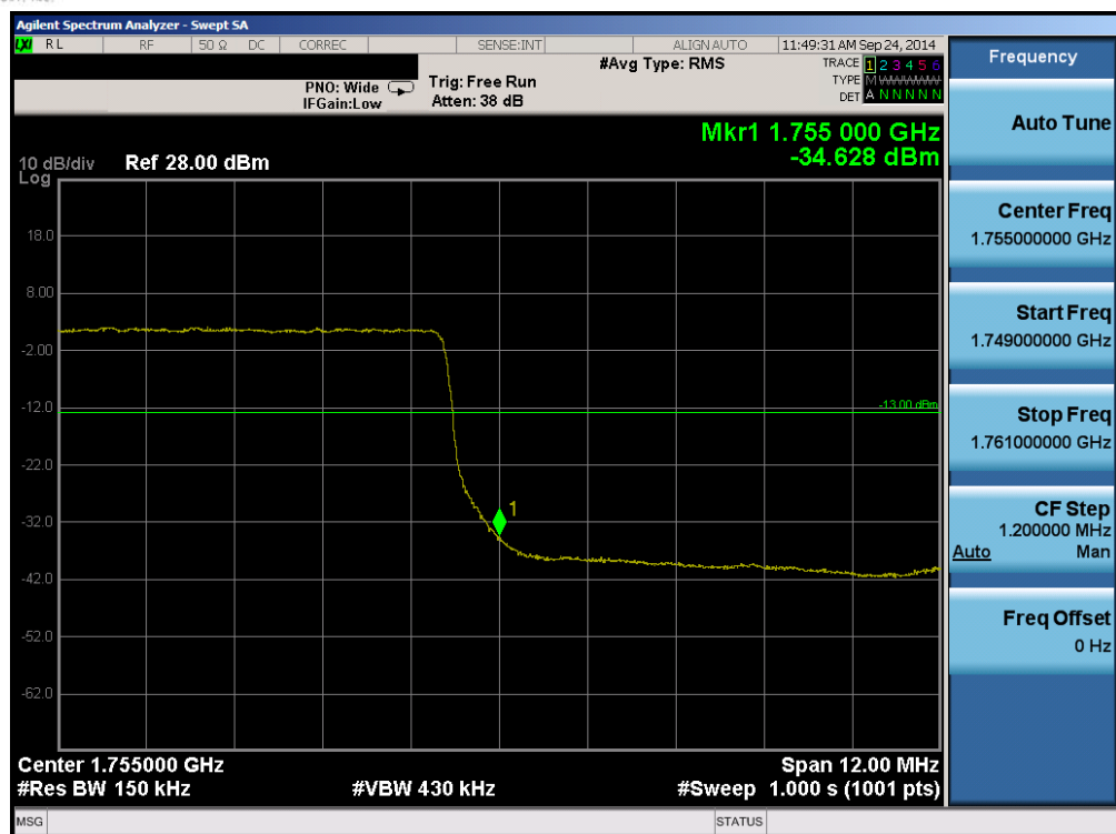
Plot 6-77. Upper Band Edge Plot (Band 4 – 15.0MHz QPSK – RB Size 75)
