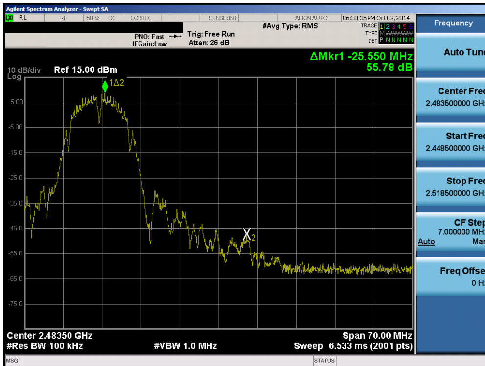
Plot 6-88. Band Edge Plot (802.11b – Ch. 11)
