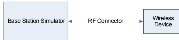
Figure 9-1 Power Measurement Setup
