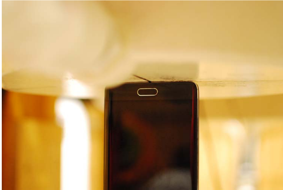
SAR Test Setup Photo 21 – Bottom Edge at 0.0 cm, Standard Cover
