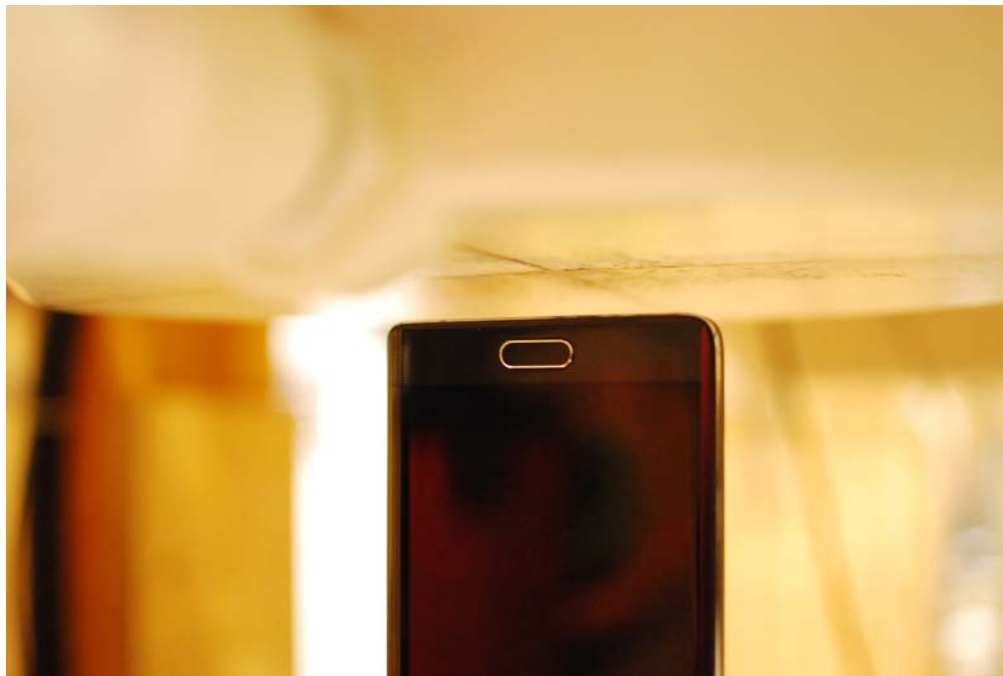
SAR Test Setup Photo 20- Bottom Edge at 1.0 cm, Wireless Charging Cover
