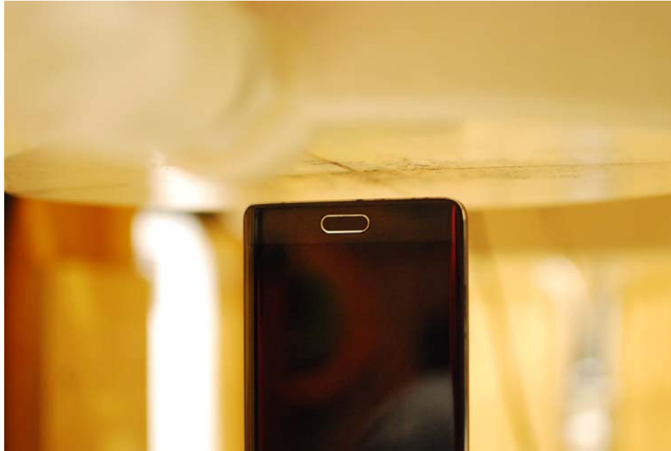
SAR Test Setup Photo 19 – Bottom Edge at 1.0 cm, Standard Cover
