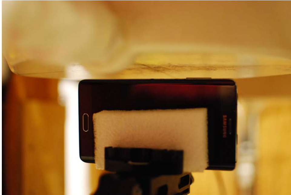
SAR Test Setup Photo 25 – Left Edge at 1.0 cm, Standard Cover
