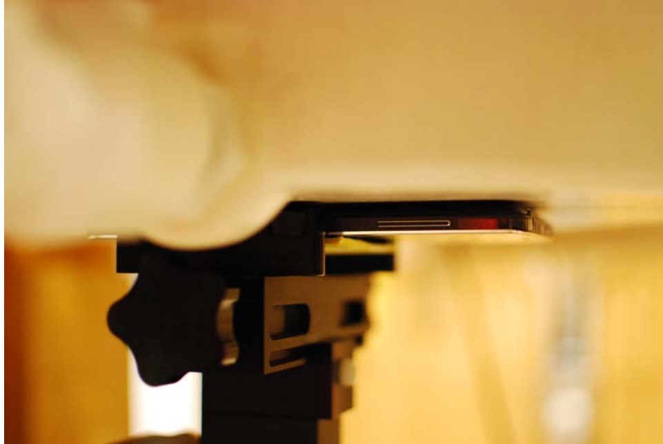
SAR Test Setup Photo 13- Back Edge at 0mm, Wireless Charging Cover
