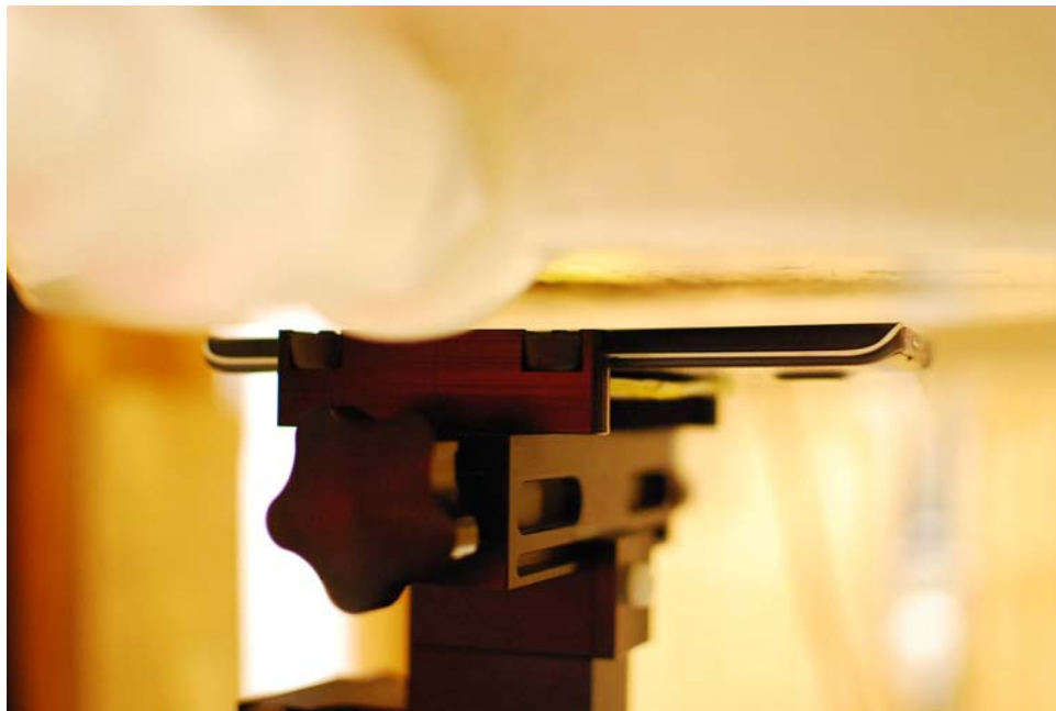
SAR Test Setup Photo 14 – Front Side at 1.0 cm, Standard Cover
