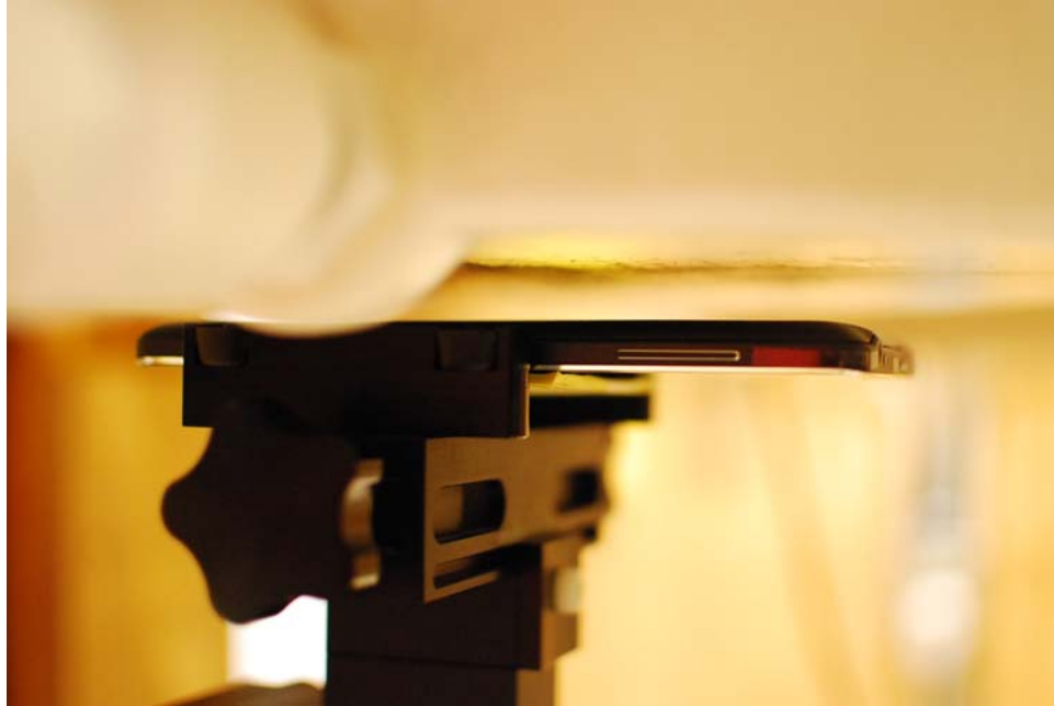
SAR Test Setup Photo 11- Back Side at 1.0 cm, Wireless Charging Cover
