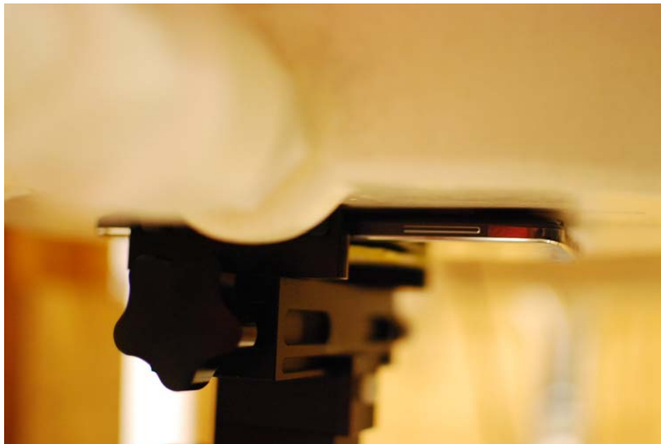
SAR Test Setup Photo 12 – Back Side at 0.0 cm, Standard Cover
