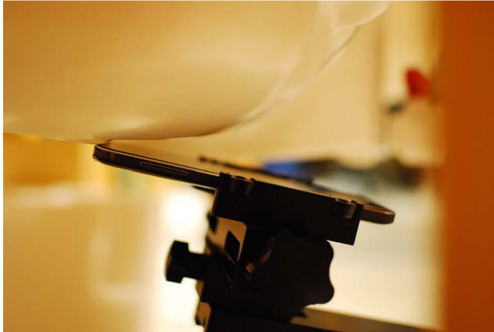
SAR Test Setup Photo 3 – Right Tilt, Standard Cover
