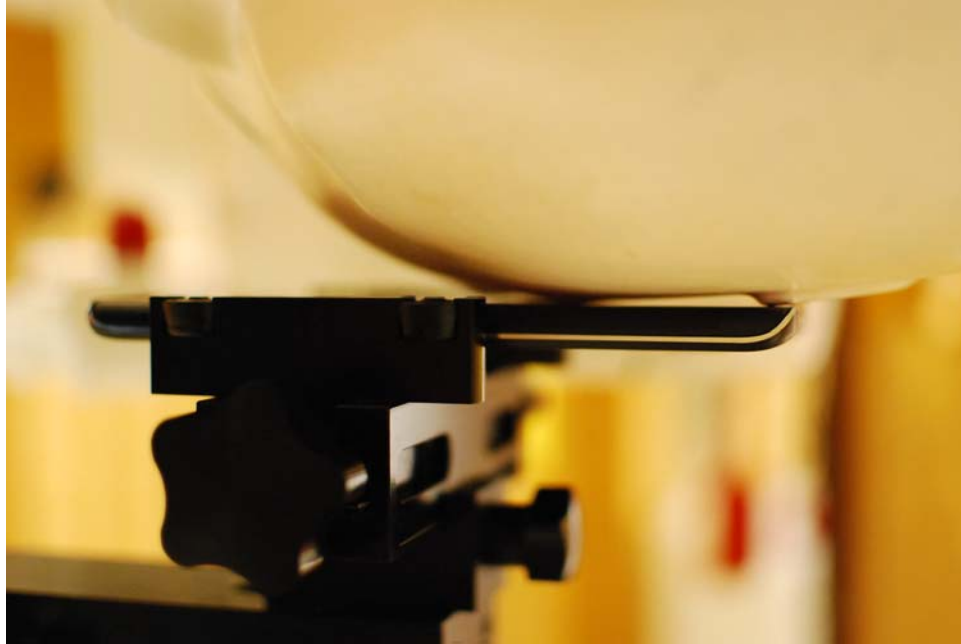
SAR Test Setup Photo 5- Left Cheek, Wireless Charging Cover
