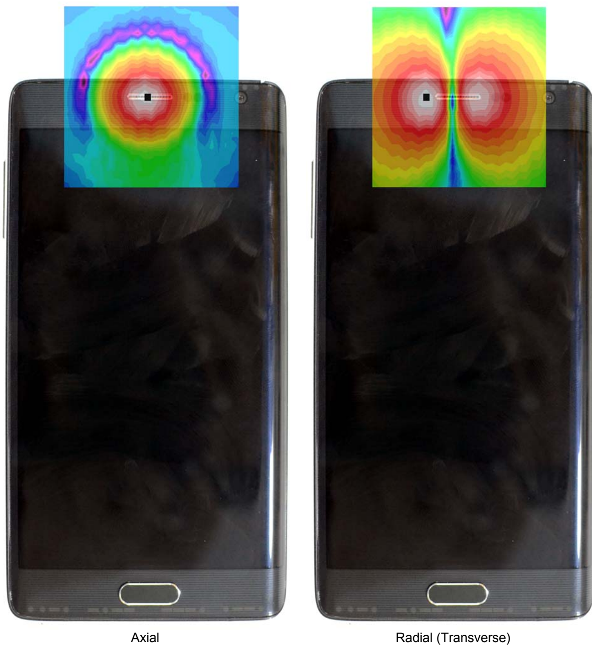
Figure 13-3 T-Coil Scan Overlay Magnetic Field Distributions
