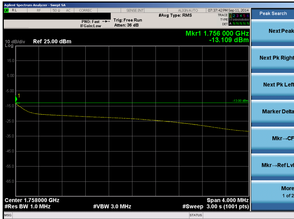
Plot 6-104. Upper Extended Band Edge Plot (Band 4 – 5.0MHz QPSK – RB Size 25)
