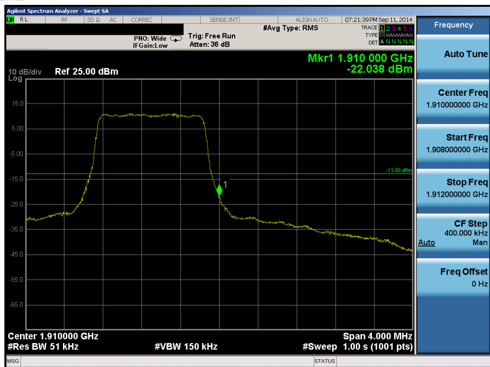
Plot 6-119. Upper Band Edge Plot (Band 2 – 1.4MHz QPSK – RB Size 6)
