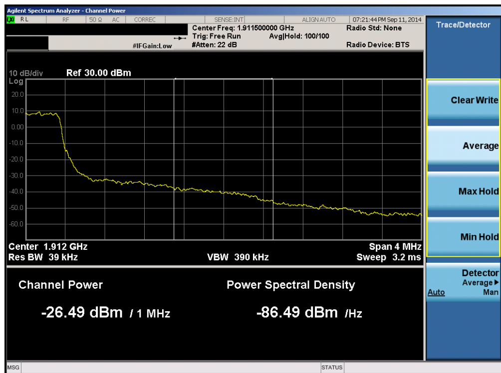
Plot 6-120. Upper Extended Band Edge Plot (Band 2 – 1.4MHz QPSK – RB Size 6)
