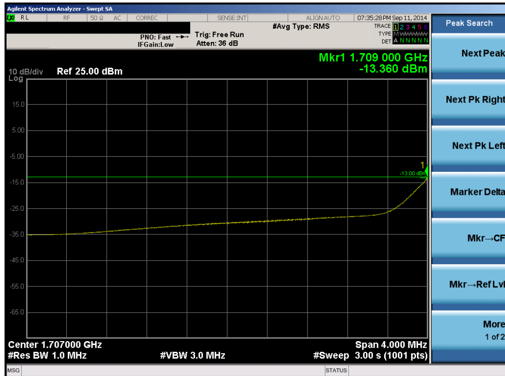
Plot 6-102. Lower Extended Band Edge Plot (Band 4 - 5.0MHz QPSK - RB Size 25)
