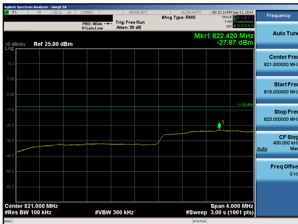
Plot 6-84. Lower Extended Band Edge Plot (Band 5 – 3.0MHz QPSK – RB Size 15)
