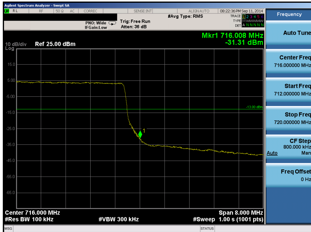
Plot 6-78. Upper Band Edge Plot (Band 12 – 10.0MHz QPSK – RB Size 50)
