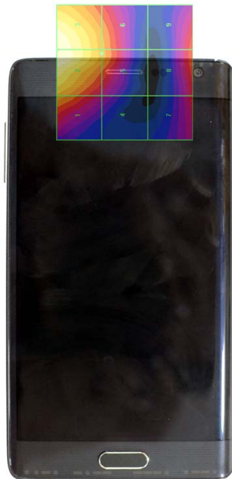
Figure 18-4 E-Field WD Scan overlay
