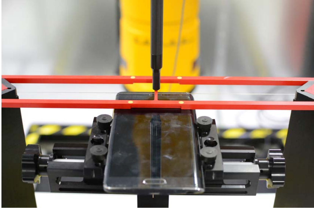
Figure 18-1 Ear Reference Point HAC Phantom Alignment
