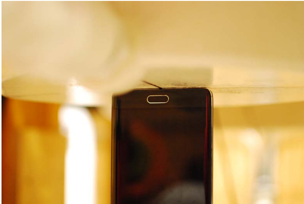
SAR Test Setup Photo 22: Bottom Edge at 0mm, Standard Back Cover
