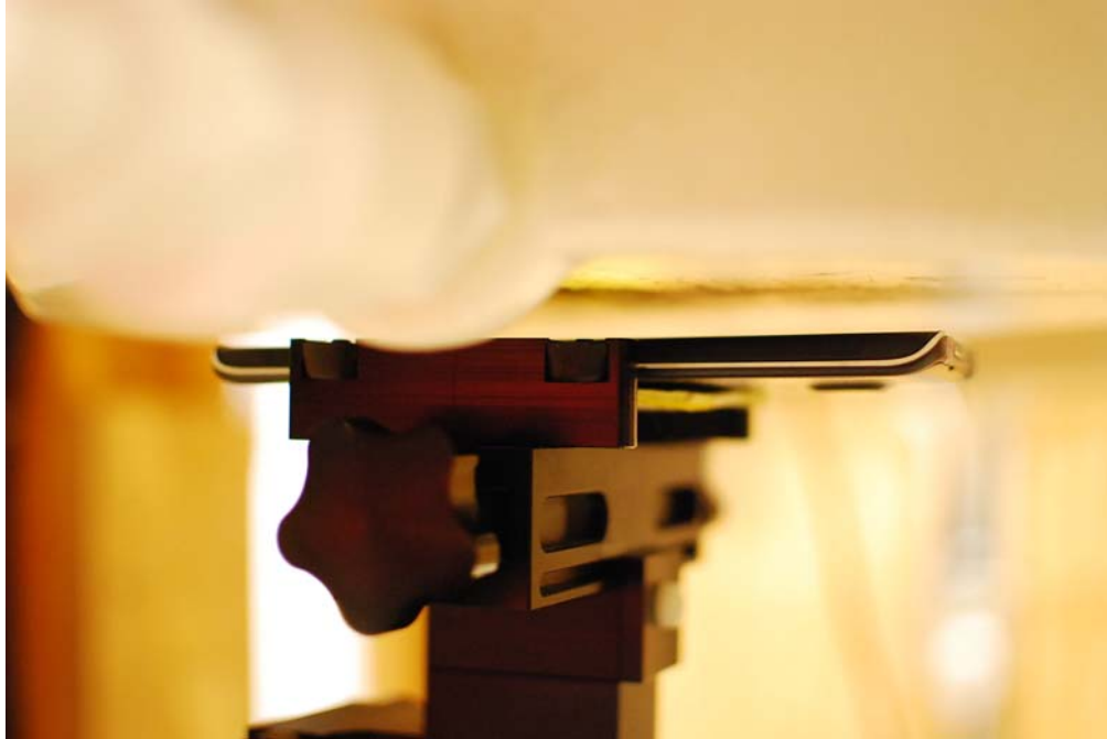
SAR Test Setup Photo 11: Front Side at 10mm, Standard Back Cover
