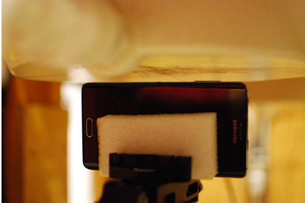
SAR Test Setup Photo 17: Left Edge at 10mm, Standard Back Cover
