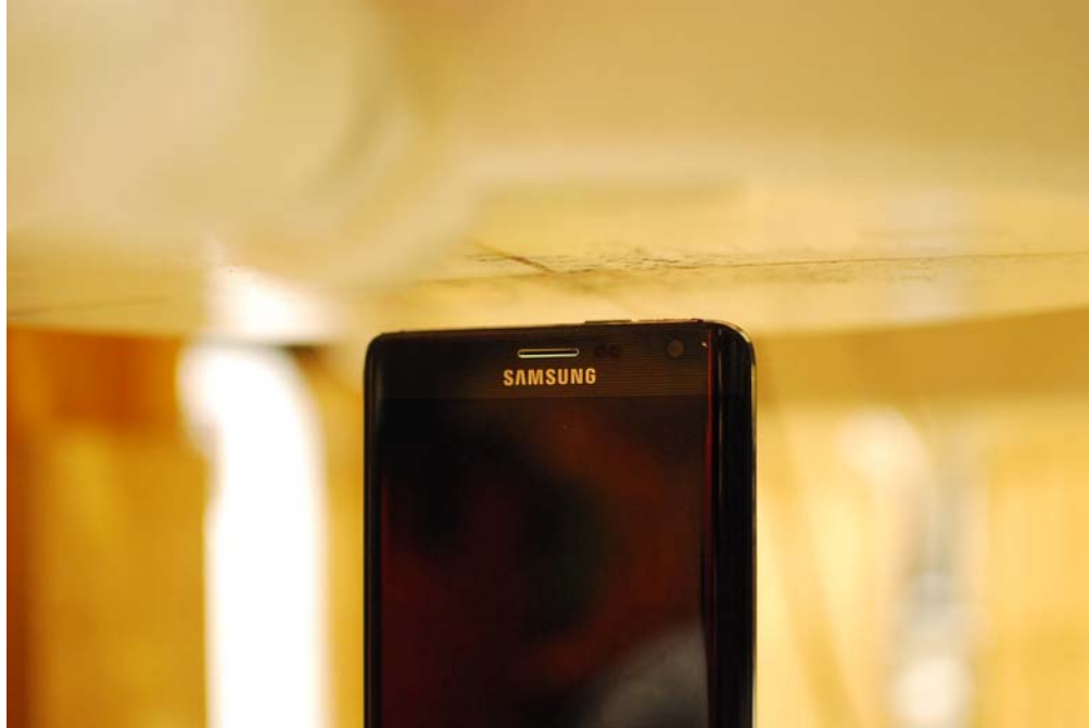
SAR Test Setup Photo 13: Top Edge at 10mm, Standard Back Cover
