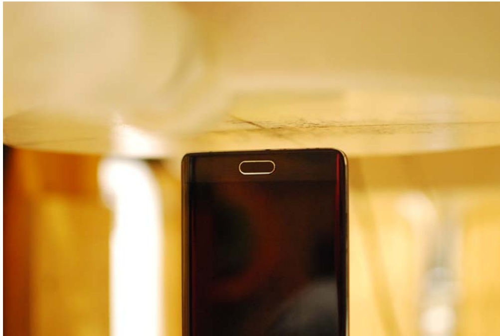
SAR Test Setup Photo 14: Bottom Edge at 10mm, Standard Back Cover
