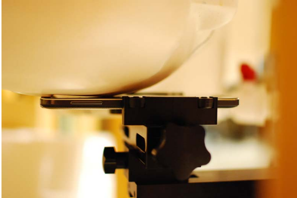
SAR Test Setup Photo 1: Right Cheek, Standard Back Cover
