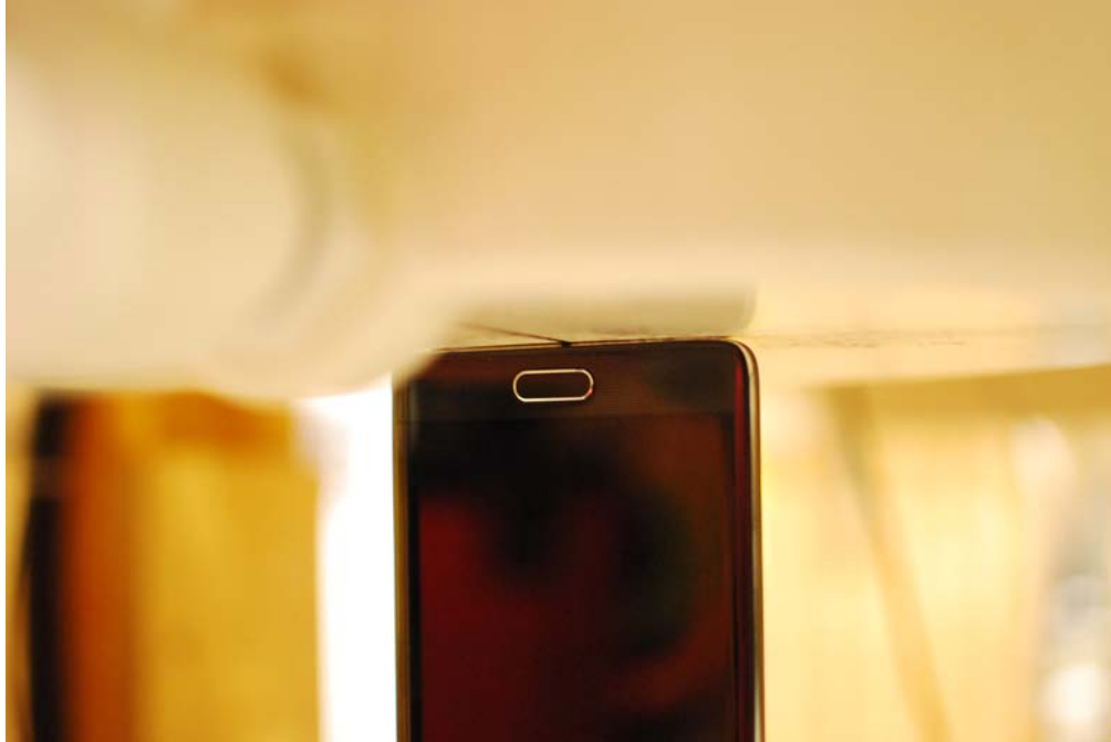
SAR Test Setup Photo 23: Bottom Edge at 0mm, Wireless Charging Cover
