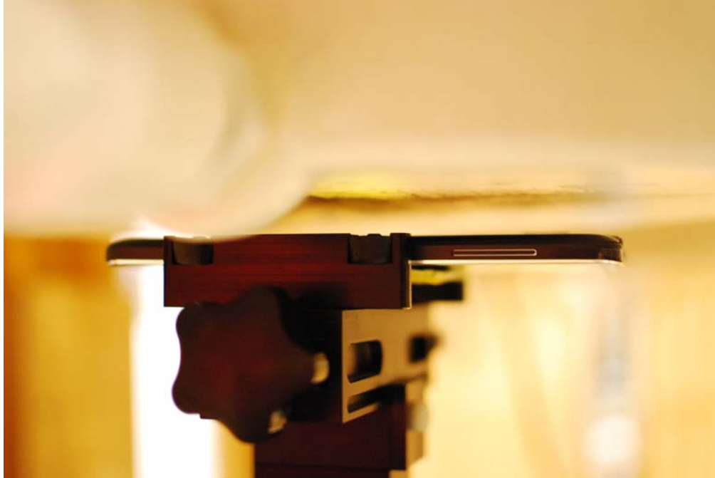
SAR Test Setup Photo 9: Back Side at 10mm, Standard Back Cover
