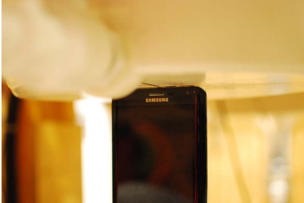
SAR Test Setup Photo 21: Top Edge at 0mm, Standard Back Cover
