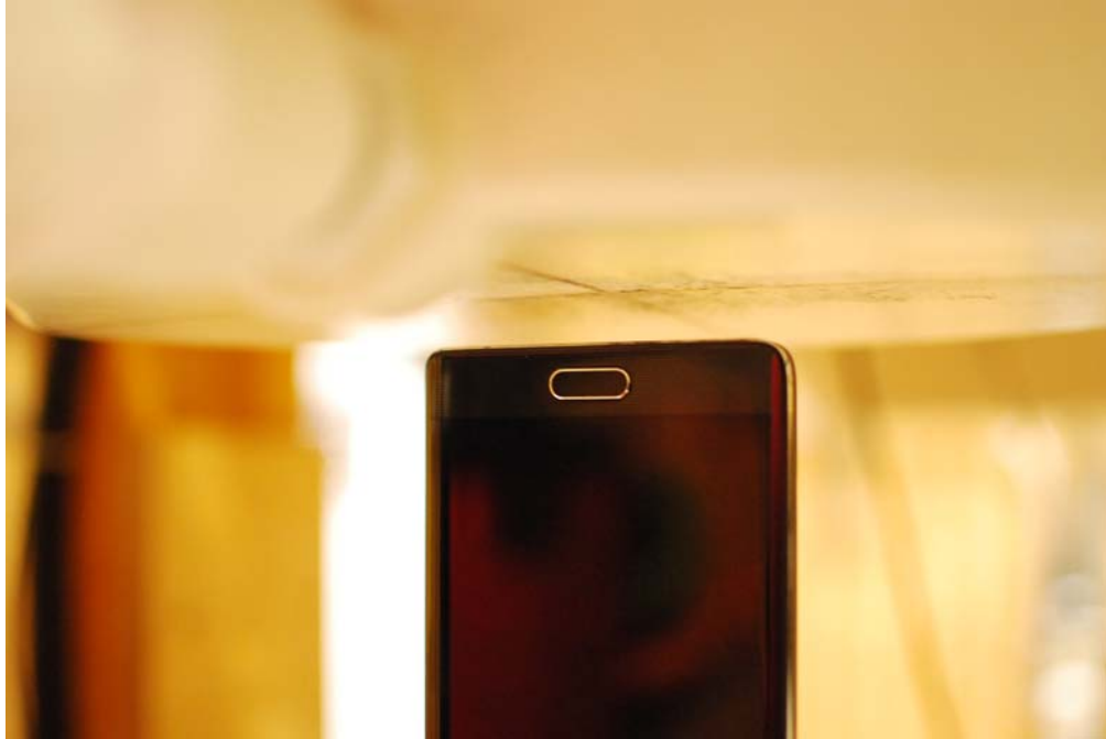
SAR Test Setup Photo 15: Bottom Edge at 10mm, Wireless Charging Cover
