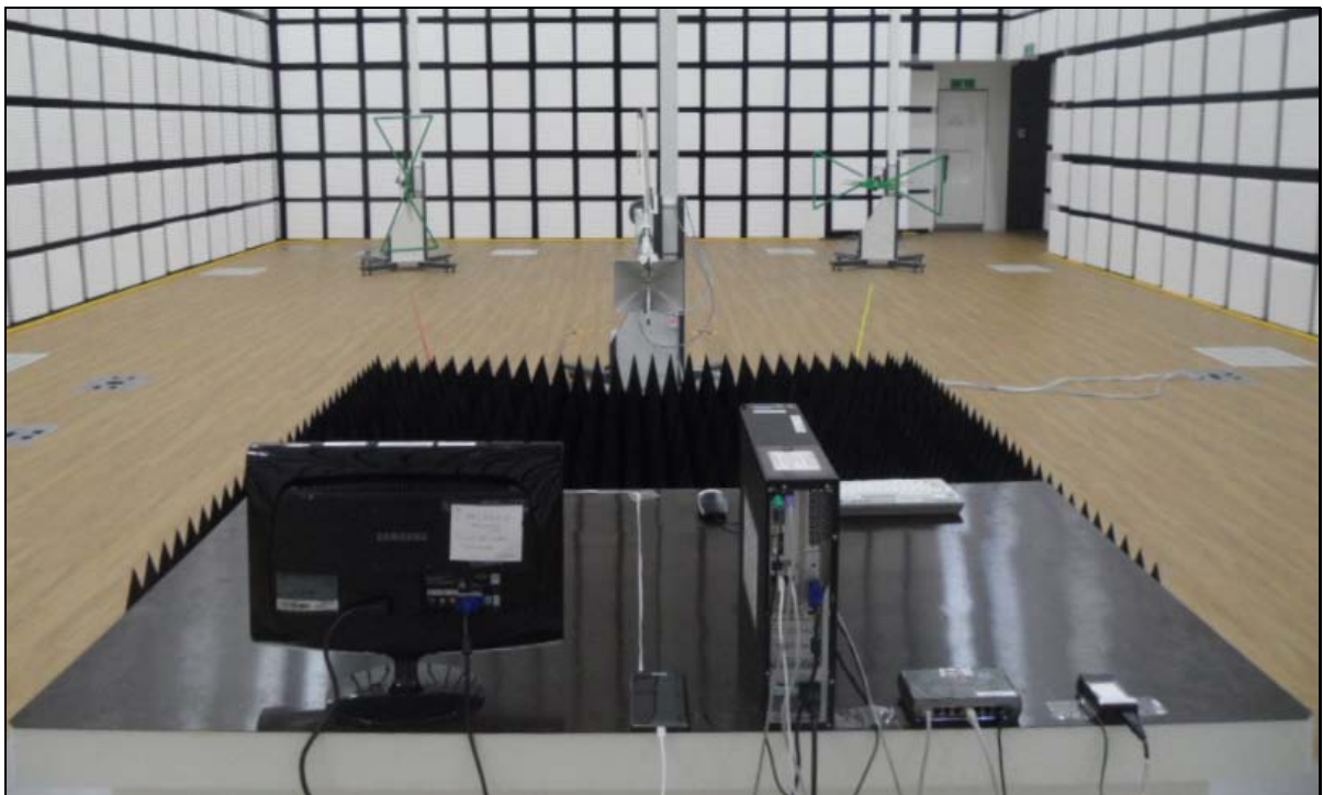
[ Radiated Disturbance for Above 1 GHz – Rear ]
