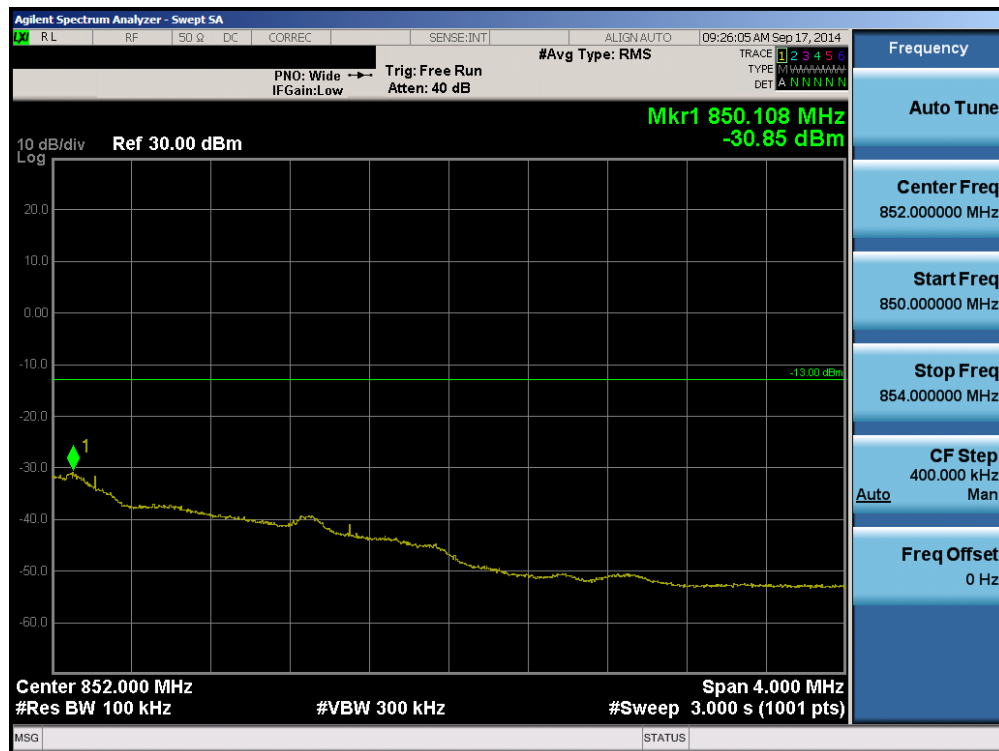
Plot 6-55. 4MHz Span Plot (Cellular CDMA Mode – Ch. 777)
