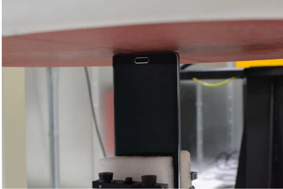
SAR Test Setup Photo 23 – Bottom Edge at 0.0 cm
