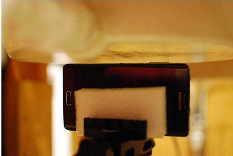
SAR Test Setup Photo 27 – Left Edge at 1.0 cm
