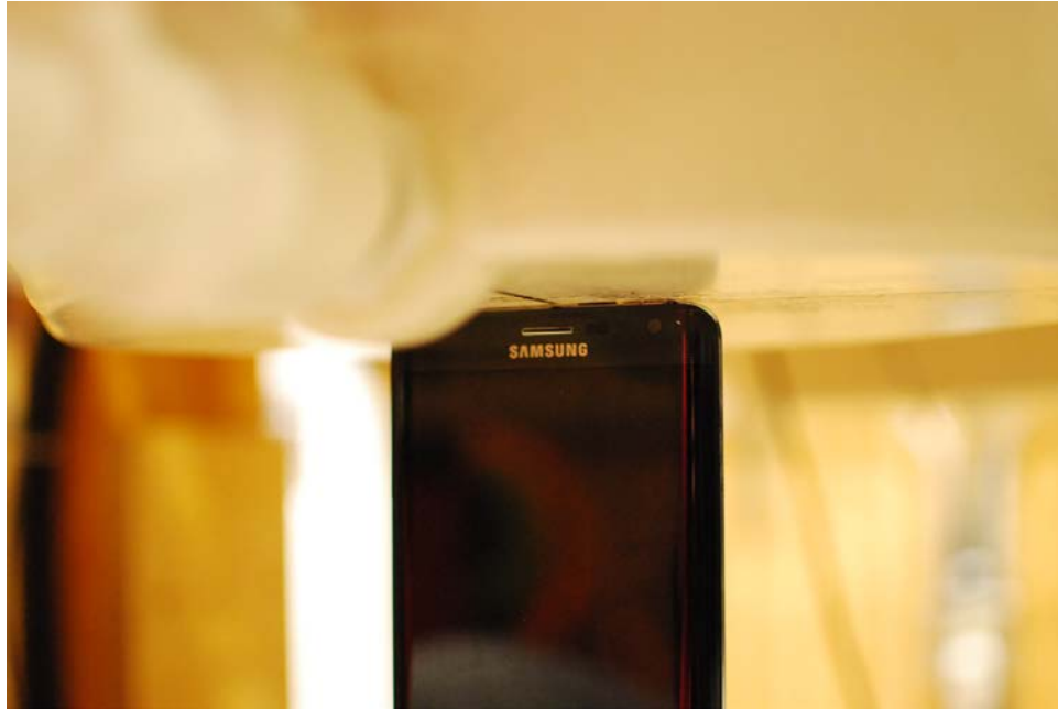
SAR Test Setup Photo 19 – Top Edge at 0.0 cm
