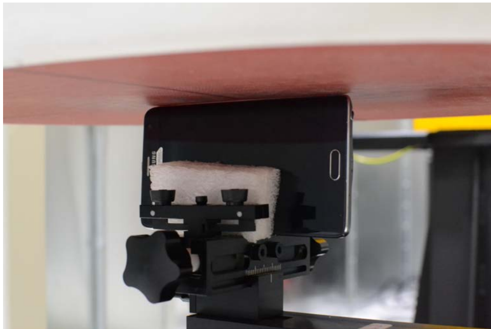
SAR Test Setup Photo 26 – Right Edge at 0.0 cm
