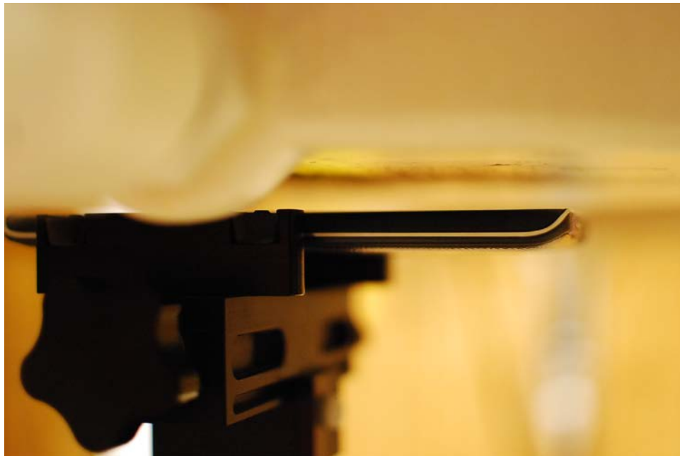
SAR Test Setup Photo 14 – Front Side at 1.0 cm with Wireless Charging Cover
