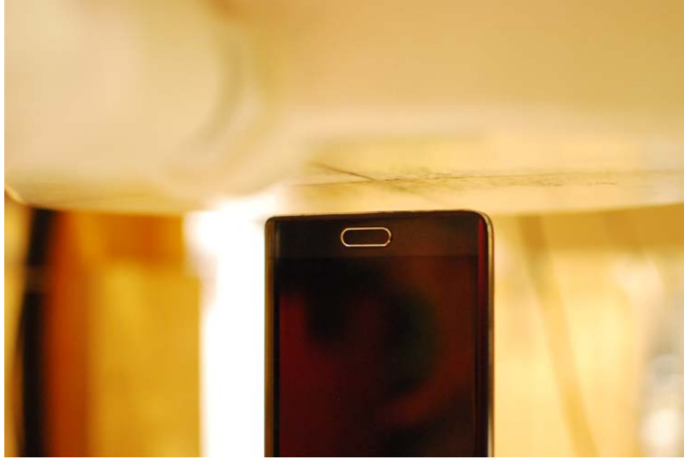
SAR Test Setup Photo 21 – Bottom Edge at 1.0 cm with Wireless Charging Cover
