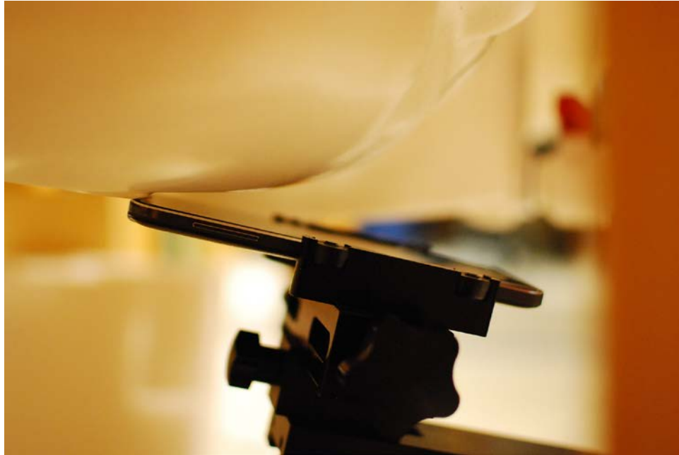
SAR Test Setup Photo 3 – Right Tilt
