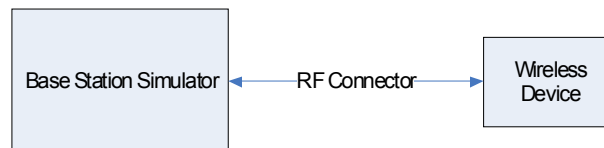
Figure 9-1 Power Measurement Setup
