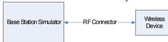
Figure 9-3 Power Measurement Setup
