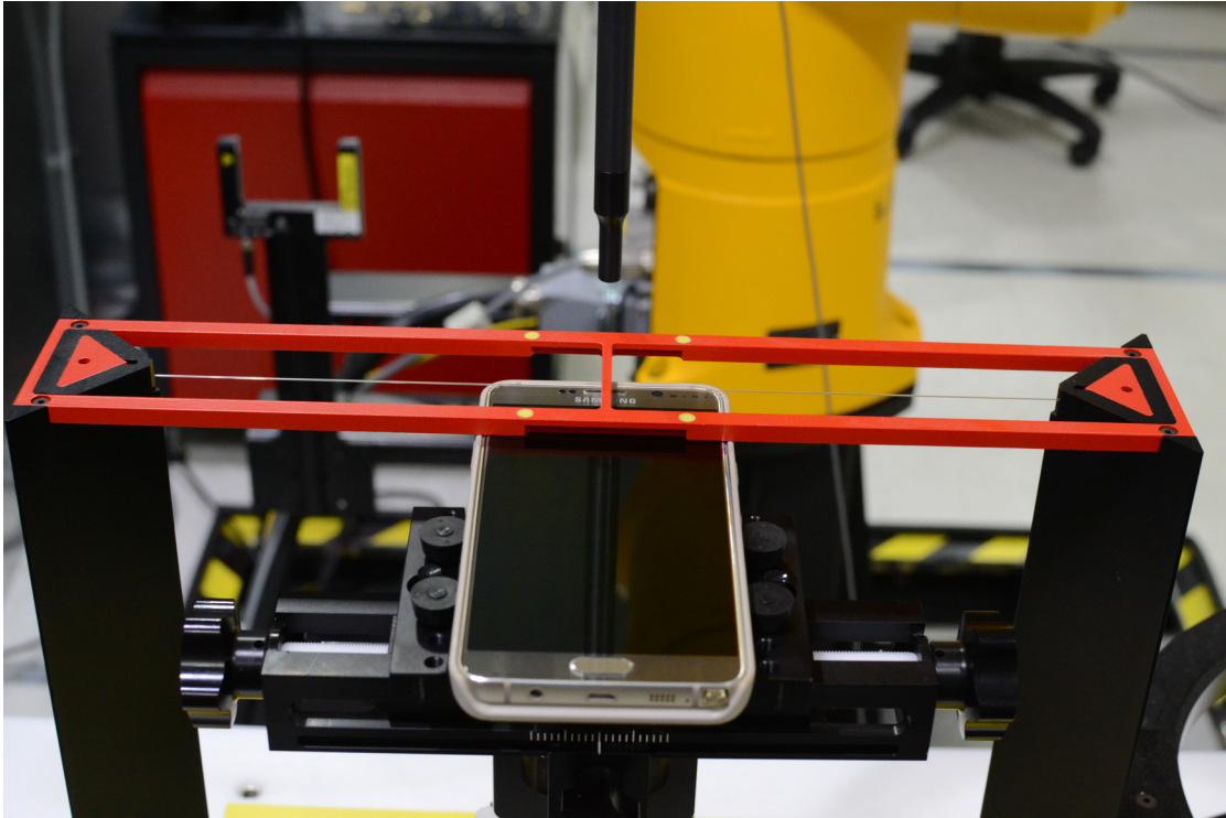
Figure 15-1 Ear Reference Point HAC Phantom Alignment
