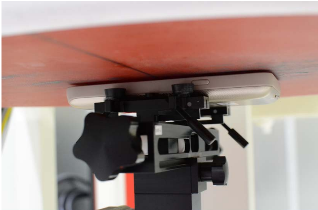
SAR Test Setup Photo 8— Front Side at 0.1 cm (Hotspot)
