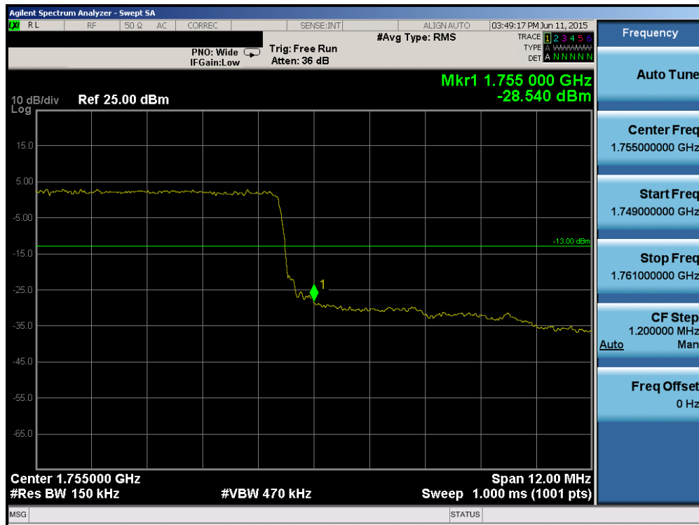
Plot 6-127. Upper Band Edge Plot (Band 4 – 15.0MHz QPSK – RB Size 75)
