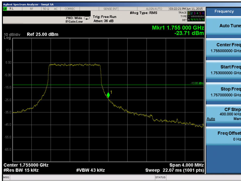
Plot 6-111. Upper Band Edge Plot (Band 4 – 1.4MHz QPSK – RB Size 6)
