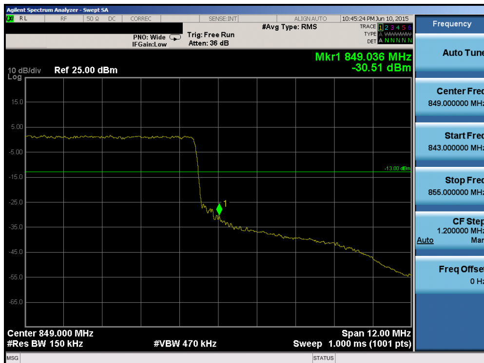
Plot 6-108. Upper Band Edge Plot (Band 26 – 15.0MHz QPSK – RB Size 75)
