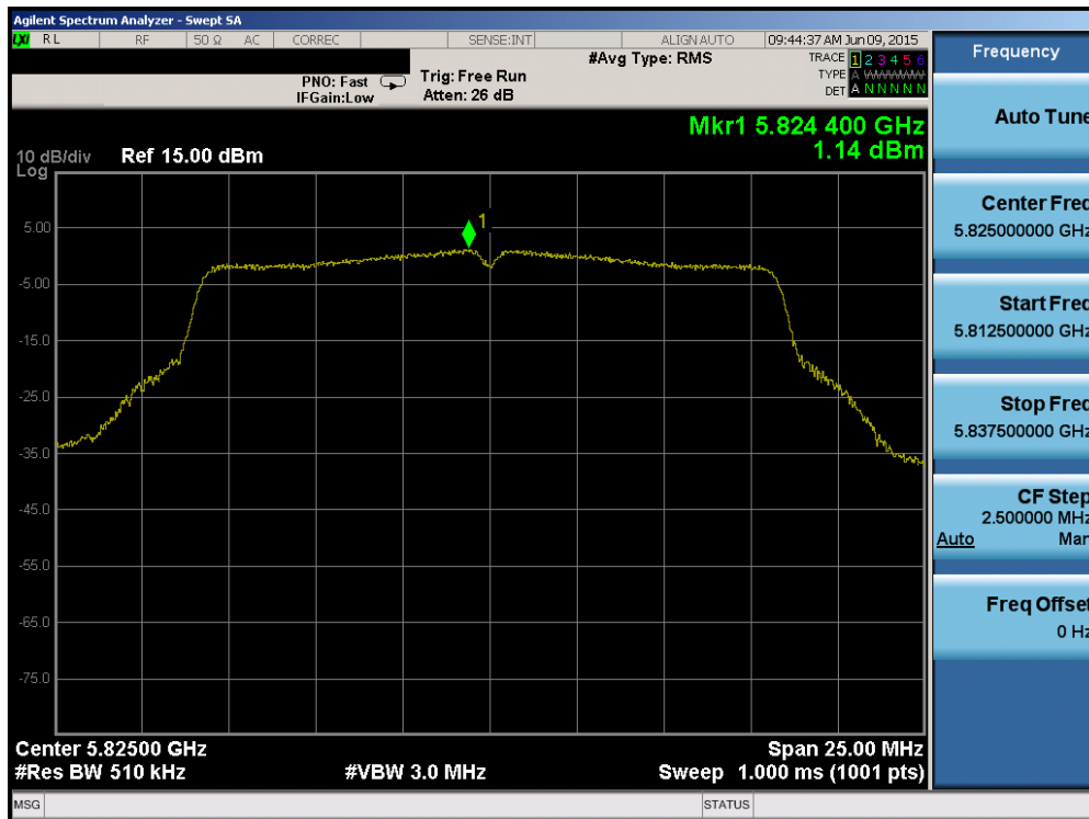
Plot 6-146. Power Spectral Density Plot (802.11a (UNII Band 3) – Ch. 165)
