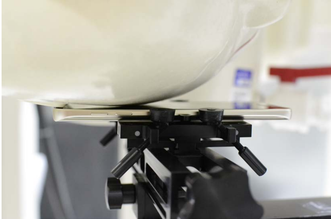
SAR Test Setup Photo 1 - Right Cheek
