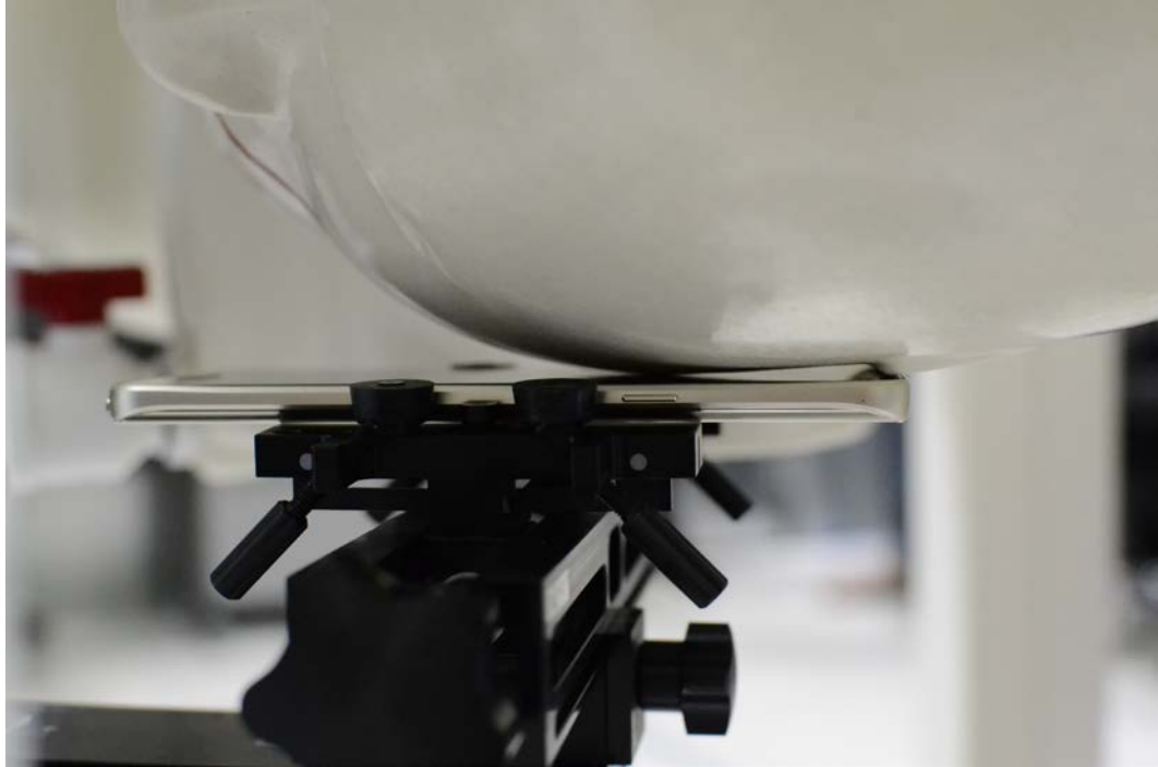
SAR Test Setup Photo 3- Left Cheek
