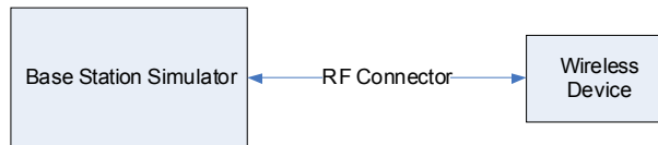
Figure 9-1 Power Measurement Setup
