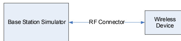
Figure 9-2 Power Measurement Setup
