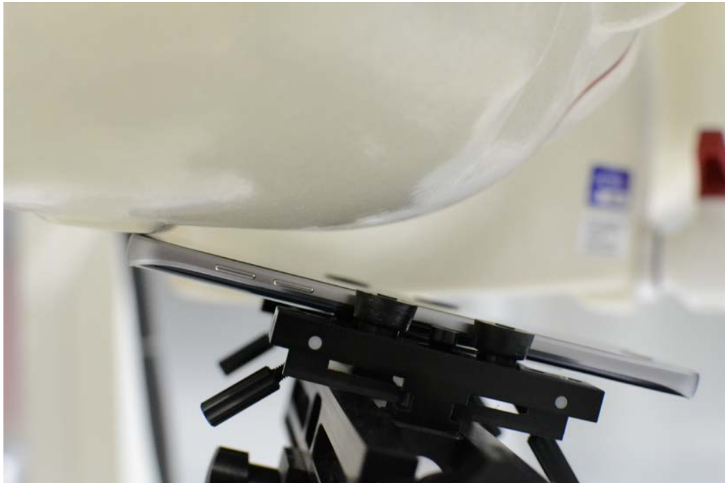
SAR Test Setup Photo 2- Right Tilt
