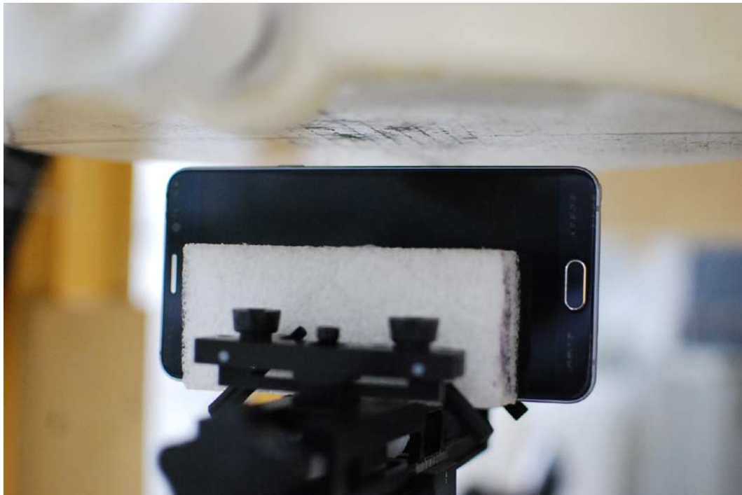
SAR Test Setup Photo 12– Right Edge at 1.0 cm (Hotspot)
